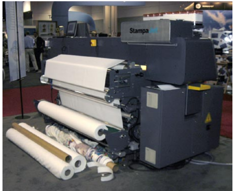
Although the printer is totally enclosed, it does not need an exhaust system. As you can see, the whole roll-to-roll mechanism is exposed.
