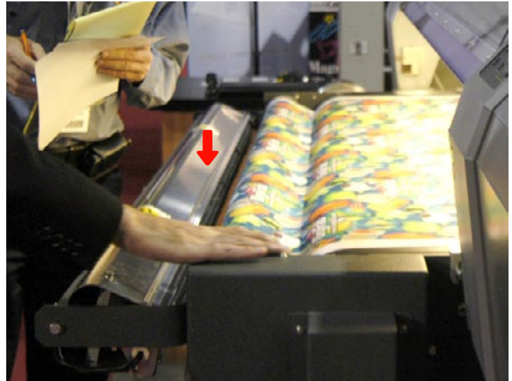
The drying unit is at the front, so that the fabric is exposed to the heat after being printed on.
