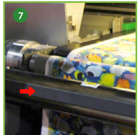
After being printed on, the fabric is exposed to the drying unit. This ensures your material won't have ink migration while being collected by the take-up unit.
