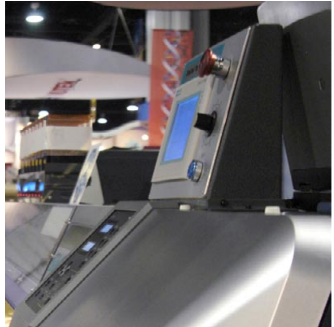
The main control area has both physical buttons and touch screen system.
