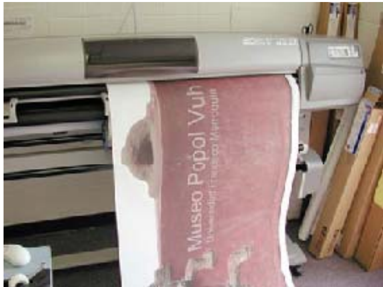
Printing a 9 foot long exhibit print on cotton from 3P Inkjet Textiles on the HP 5000ps with UV pigmented inks, FLAAR studio on the campus of BGSU.
