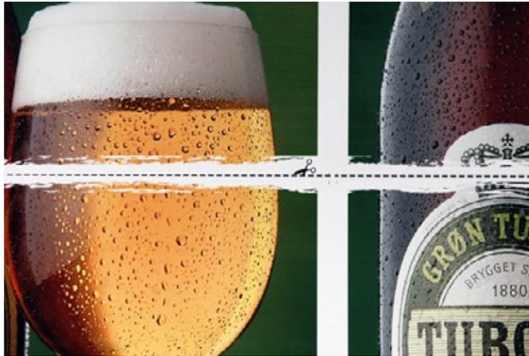
*At the top, before Intelligent Interweaving is turned on; there are horizontal bands. The lower half (after the scissors), Intelligent Interweaving is turned on, and no more visible banding.*
