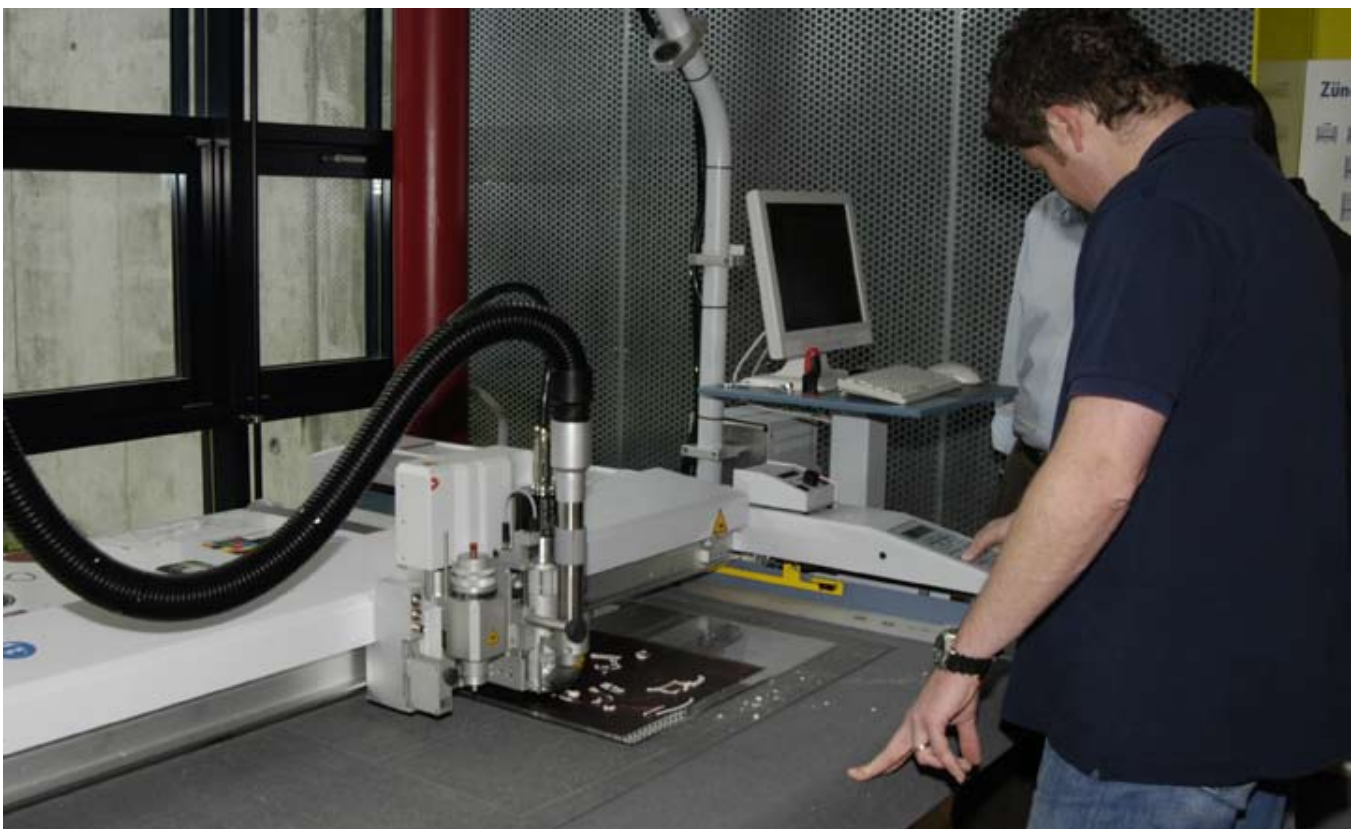
Figure 11b. Tool pressure is adjusted from the main console.
