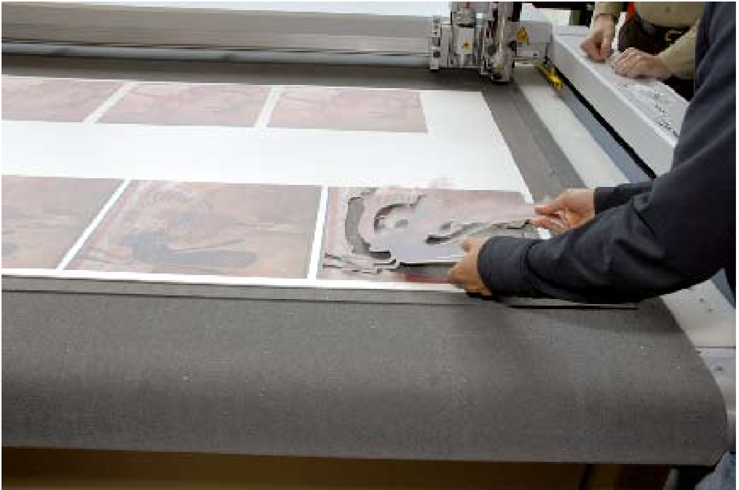
Figure 12. Dibond can also be routed.
