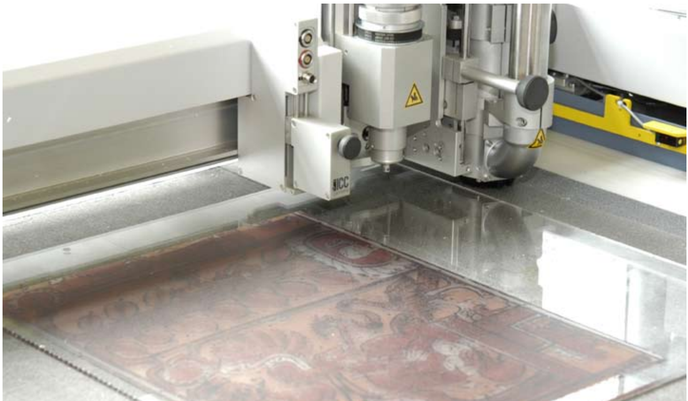
Figure 10b. Plexiglass is one of the several materials available that can be printed or cut.
