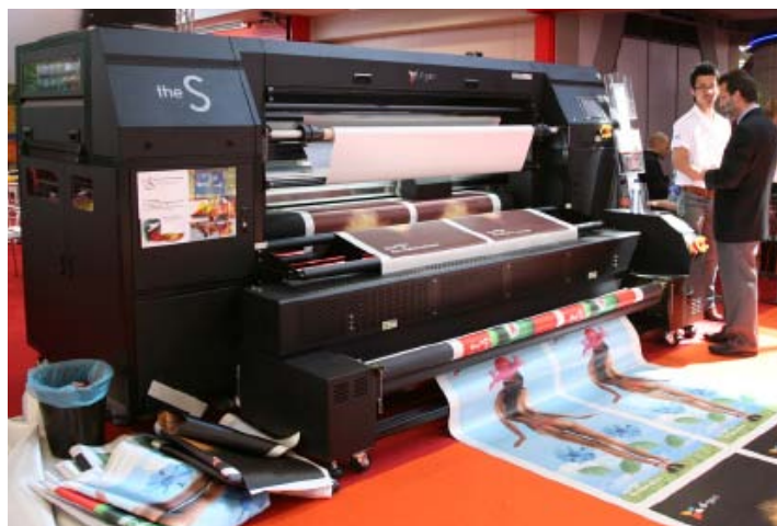
D.gen the S, prints the front and rear at the same time.
