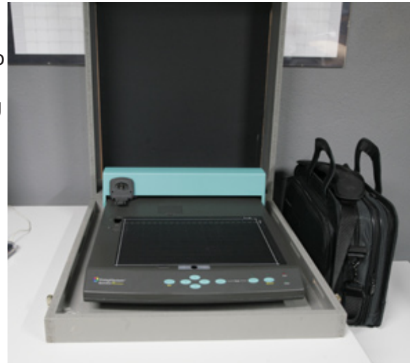
Here is a GretagMacbeth Spectrolino, the elite spectrophotometer of the last several years. Granis has built a custom-made carrying case, since he often goes out as a consultant and works on-site in other print shops. We cover color management tools and software in a separate series of FLAAR Reports, available on www.wide-format-printers.NET .
