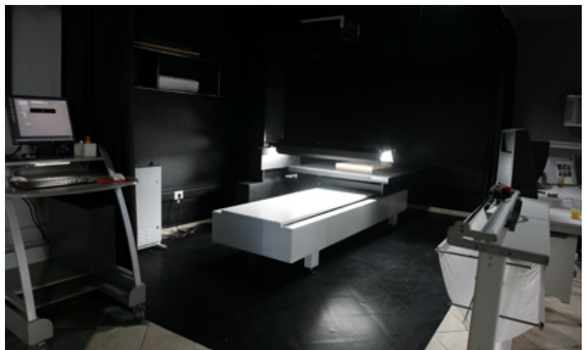
Another view of the Cruse scanner with the curtain opened so we can see the synchron table (a patented system). Although I generally use the reference as the Rolls Royce of giclee capture systems, in reality this is more like a Mack Truck; it is built the way you expect a German machine to be built like. At the right, that is a wide format trimmer, an essential piece of equipment. If you wish additional information on trimmers (and are in the USA), you can contact Mike Lind at www.reprographicdesigns.com , 281 492 2714, malind@msn.com
