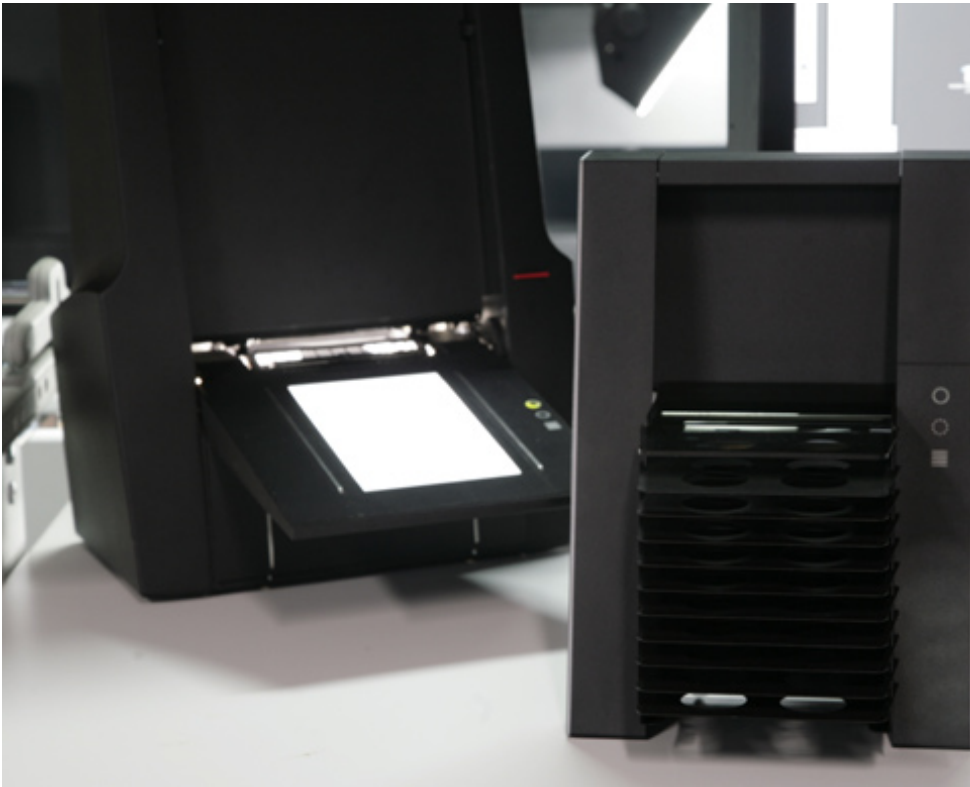
A close-up of the not-so-functional multi-side feeder. The Imacon is really made for one side at a time, each fed manually.
