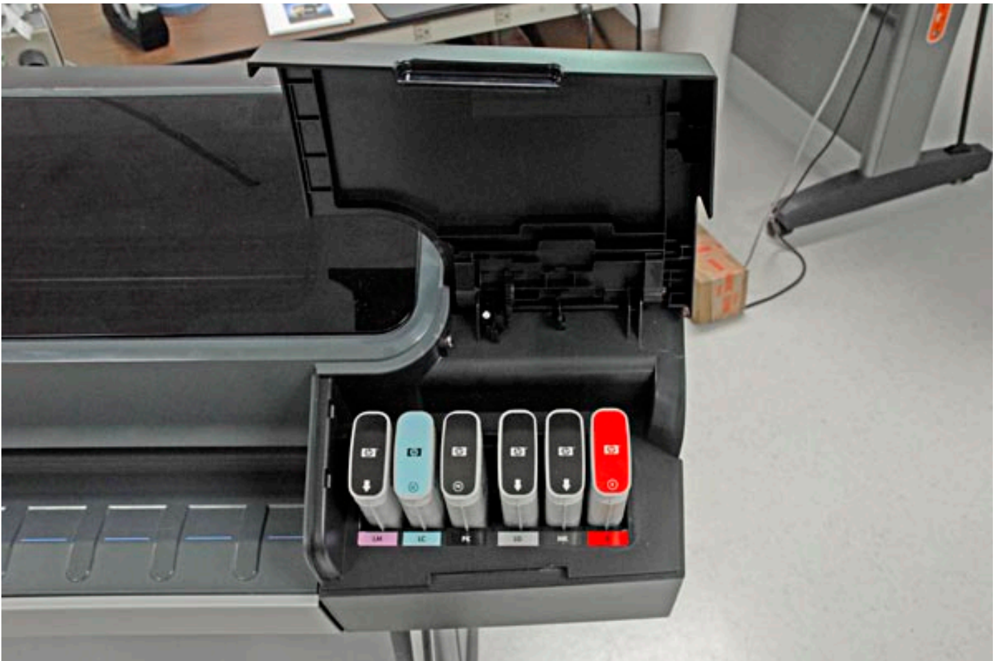
The ink containers are located at the front at each side of the printer
