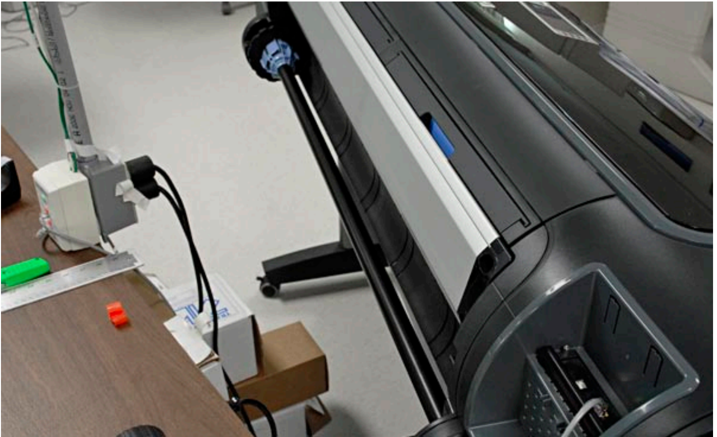
Spindle accepts a standard diameter of two inches.
