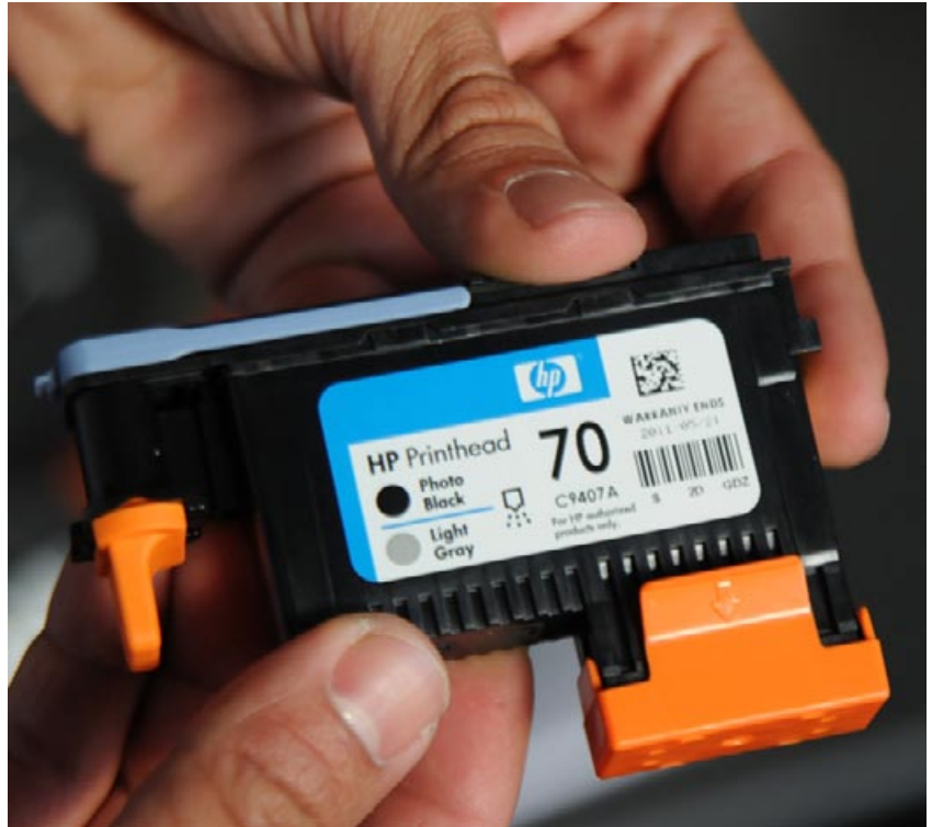
Each printhead handles two colors.
