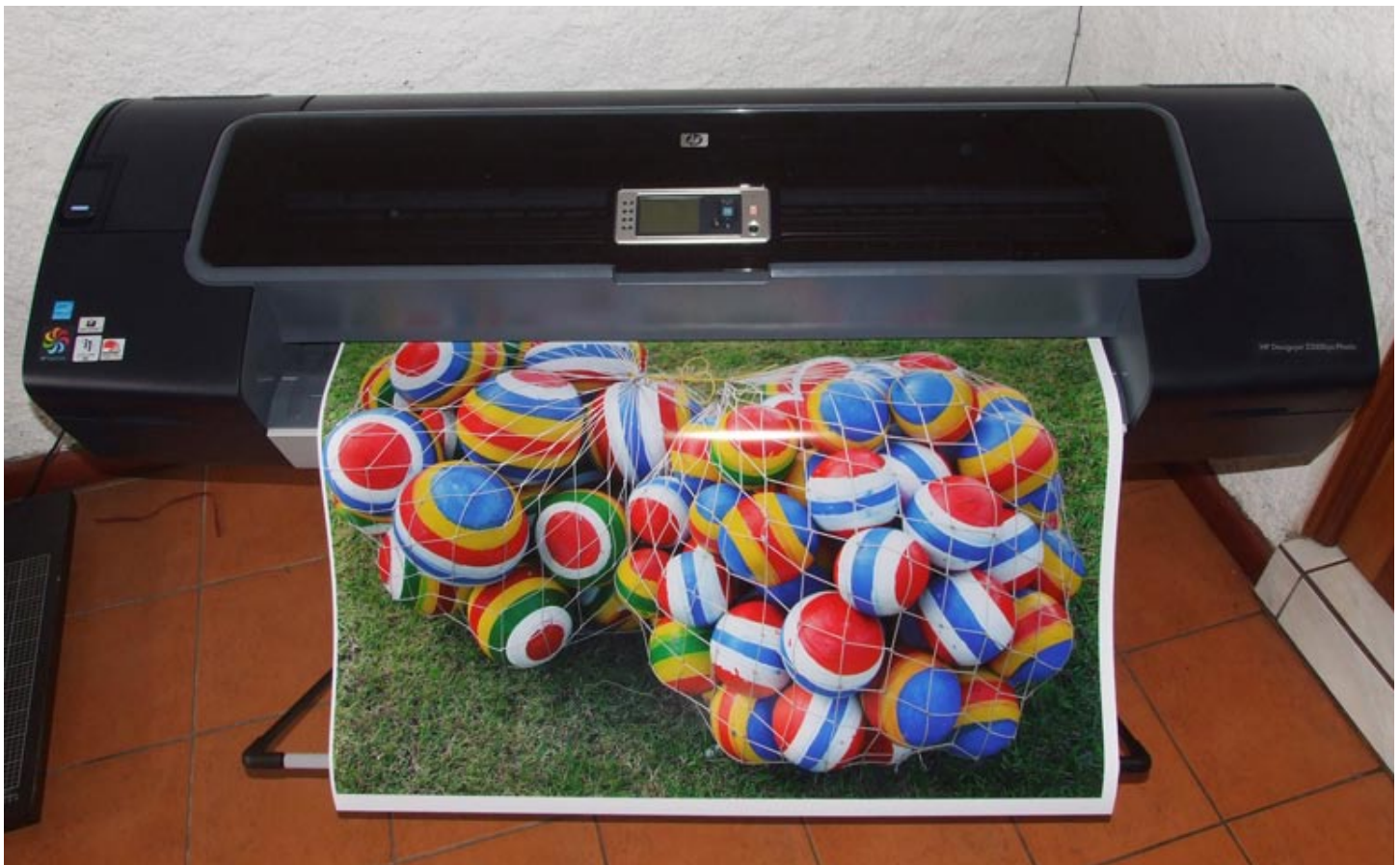
This model prints up to 44”, but there is a smaller version that prints up to 24”. The photograph being printed was taken by Nicholas Hellmuth.
