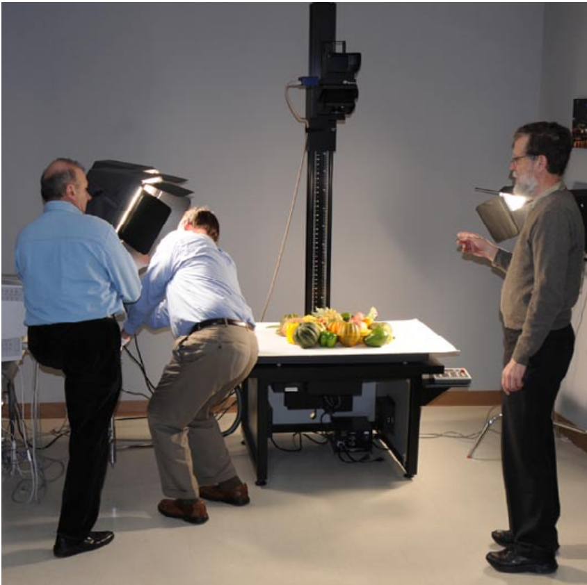
Betterlight Super 8K-HS large format scanning back.
