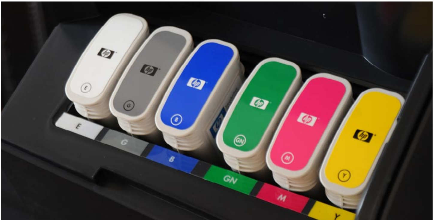
There are six cartridge slots at each side of the printer., one of which is a gloss enhancer.
