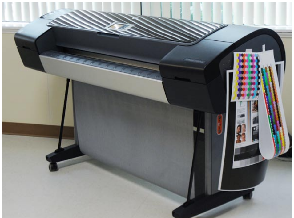
The printer comes with a wheeled stand and a basket to receive media.
