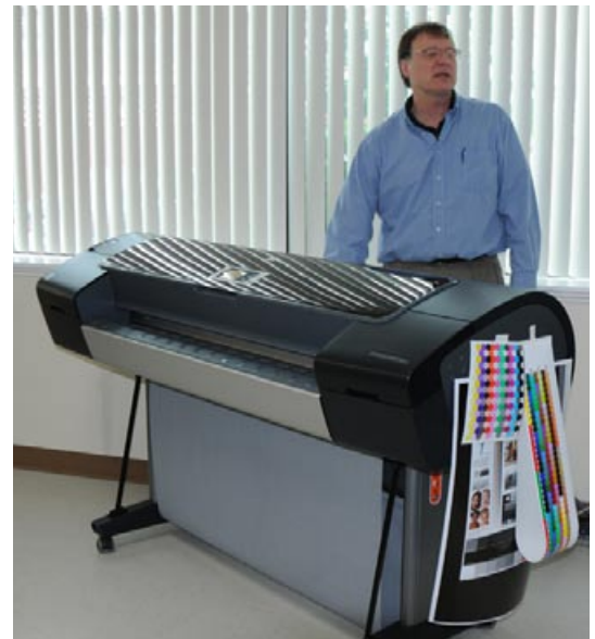
Media is loaded at the back. The instructions to properly load the roll of media were not very clear in the sense that the manual mentions lefts and rights, but it is hard to know if they mean viewed from the back or from the front. In these photos, Randy Ross, from Parrot Digigraphic loading a roll of media.
