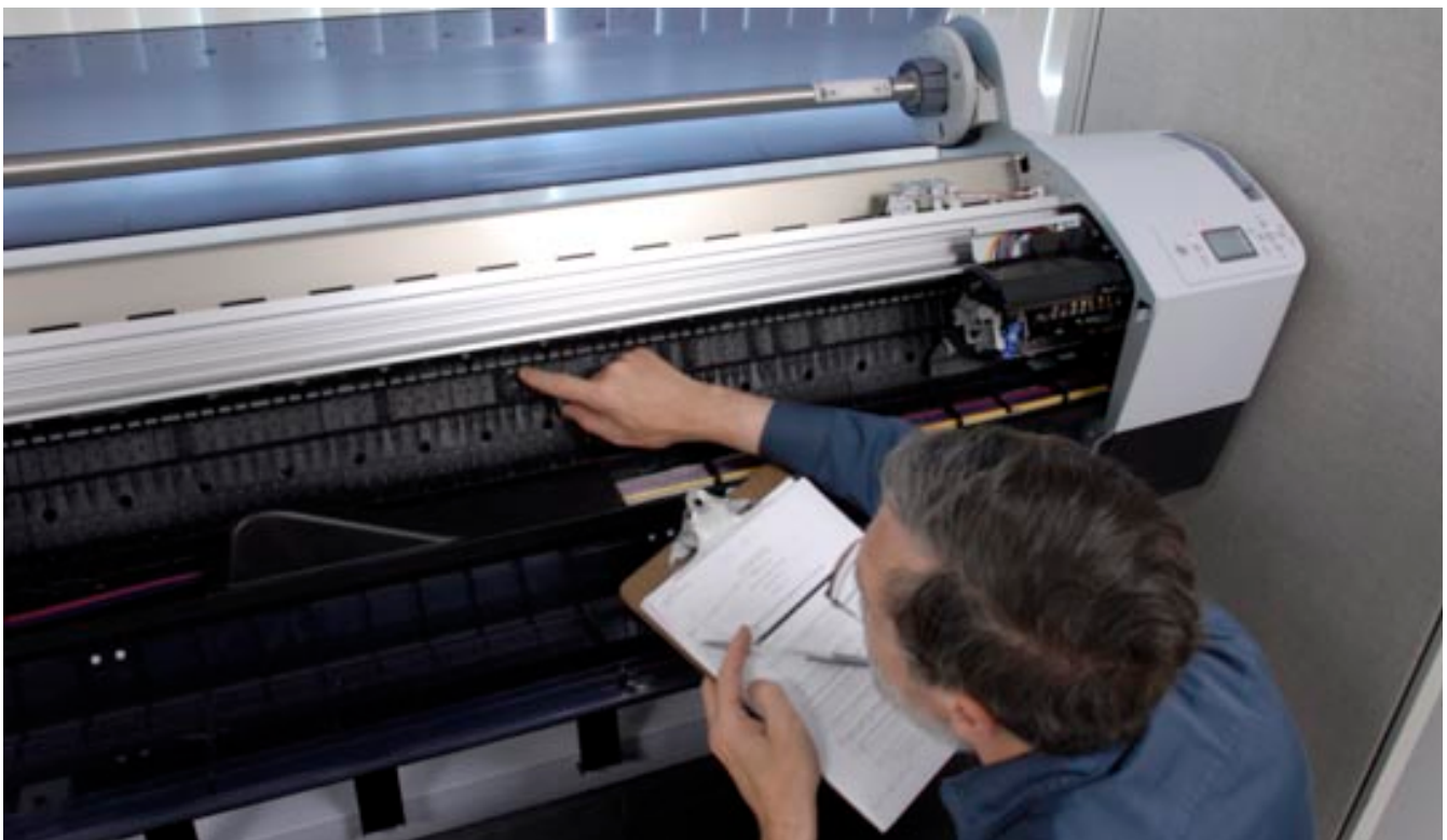
Dr. Hellmuth evaluating the carriage of the Epson Stylus 9880 printer at Parrot Digigraphic.
