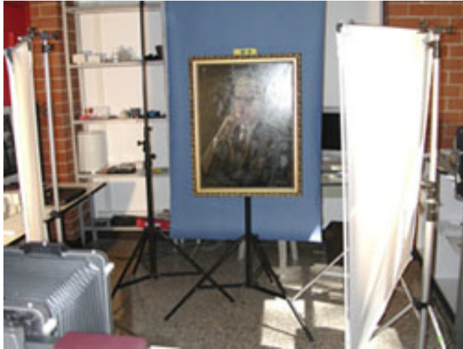
This image shows reflection of light in the painting, using Lowel Dp lights, the final picture was taken without the white cloths using Lowel Tota Tungsten lights.
