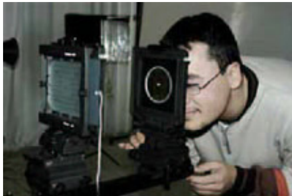
Aligning the camera standards with the Zig-Align
