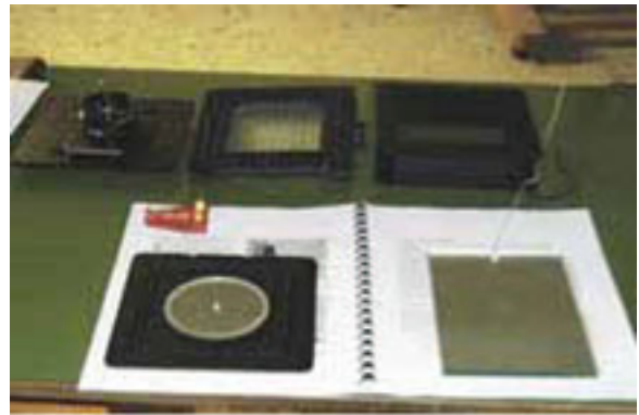
Lens, camera standard, bellow, bubble level, & Zig-align Mirror system
