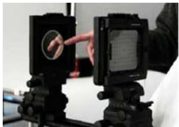
Circular mirror attached to the lensboard
