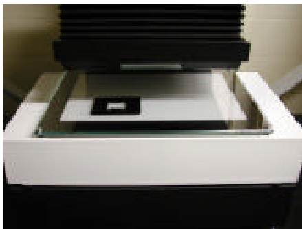
Figure 4: The light box attachment used for negatives, positives, and transparencies.
