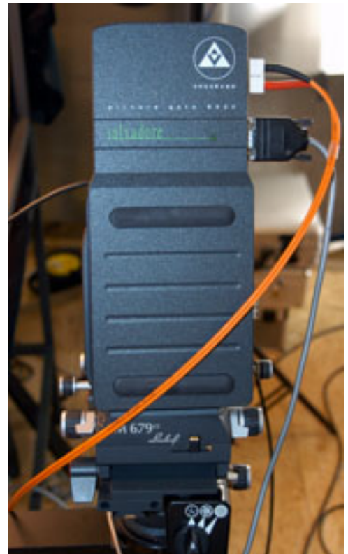
Anagramm is a large format back, here inserted into a medium format camera (the Linhof 679). This size camera is made to hold medium format backs so will cut off a few centimeters of the image area of a large format back, but a Linhof 679 camera is very handy and is a good selection for a studio-ready professional quality camera.
