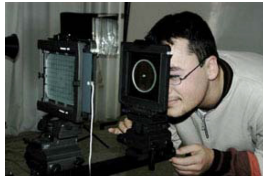
David aligning the camera standards with the Zig-Align
