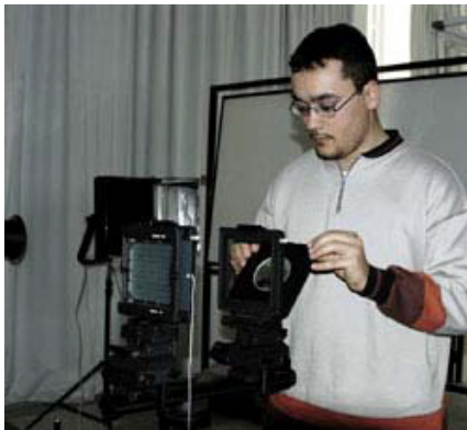
David aligning the camera standards with the Zig-Align
