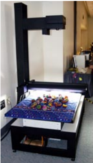
Here is a Cruse scanner in operation at Siggraph 2003, scanning some 3-dimensional objects, in this case Guatemalan handicrafts made from hand-woven textiles. You can call this either a scanner or a digital camera: the CCD is similar either way. I consider the Cruse to be a digital camera, but it uses a tri-linear scanning CCD, not a CCD in Bayer Pattern that is in a medium format or 35mm digital camera.
