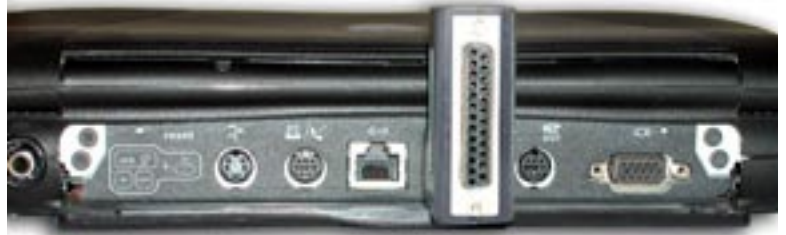
SCSI adaptor shown on the back of a Mac "Wallstreet" laptop. No recent Mac has SCSI, but you can add a card. SCSI is faster than USB and faster than most FireWire, but has a few operating quirks, such as requiring a terminator plug.
