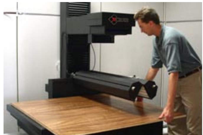
One model of Cruse scanner has lights that move in unison with the scanner head; another model of the Cruse has the transport table move in unison with the scanning mechanism.
