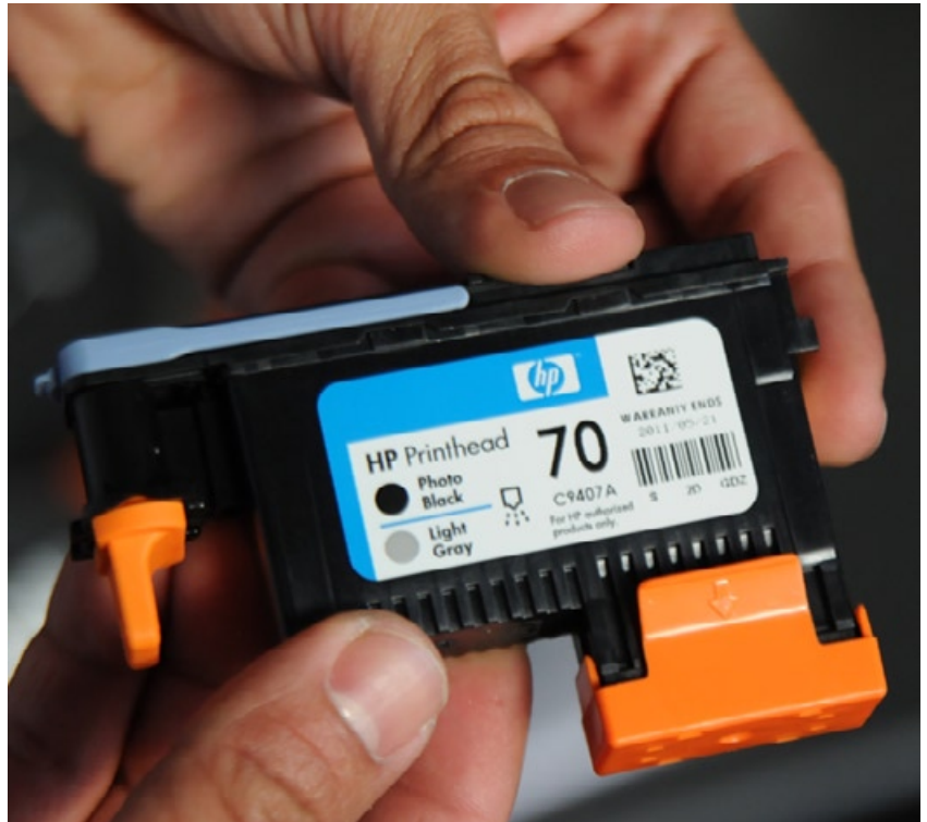
Each printhead handles two colors.
