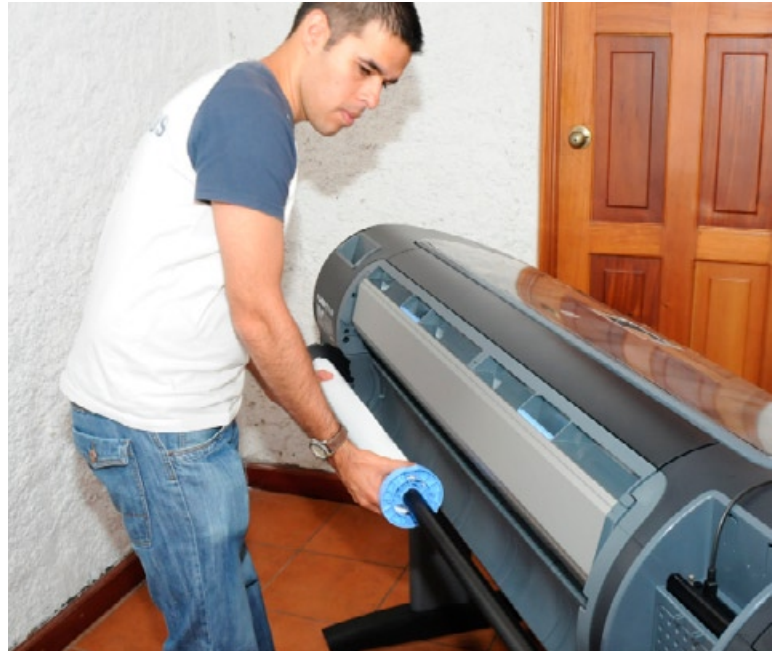
Media is loaded at the back. The instructions to properly load the roll of media were not very clear in the sense that the manual mentions lefts and rights, but it is hard to know if they mean viewed from the back or from the front.
