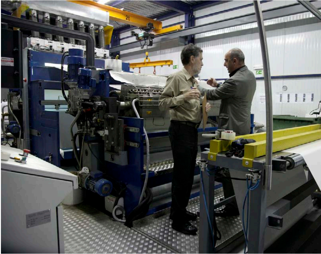
Here is Rui (DIGIDELTA) explaining the applying self-adhesive backing process to Nicholas Hellmuth.
