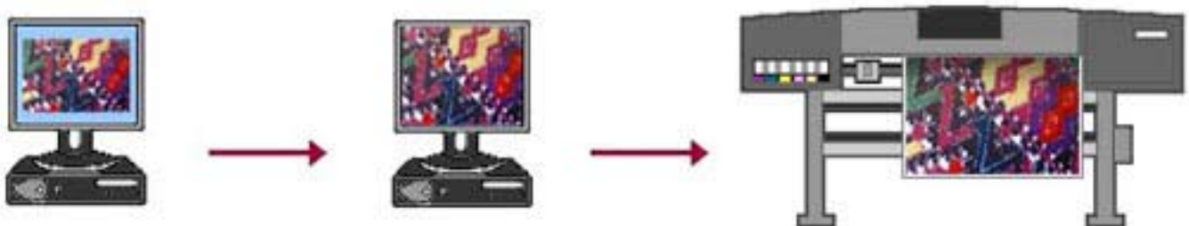
5 th workflow diagram: PC as image capture, PC as RIP station, HP 5500, this is the fastest of the solutions if the RIP can RIP on the fly.
