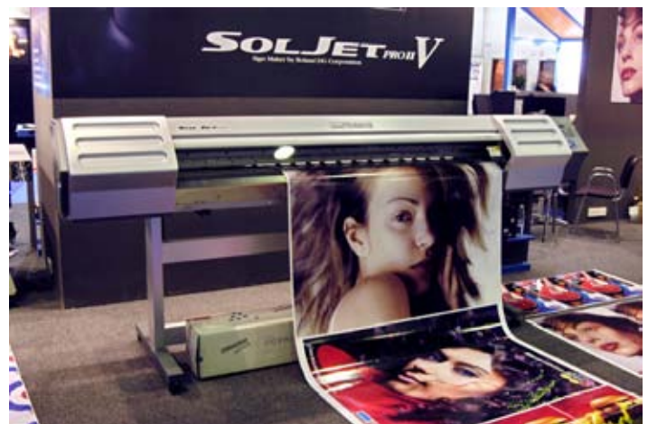
Roland Pro II at Dubai 2006. This eco-solvent printer uses Epson piezo heads which can produce up to 360 dpi.
