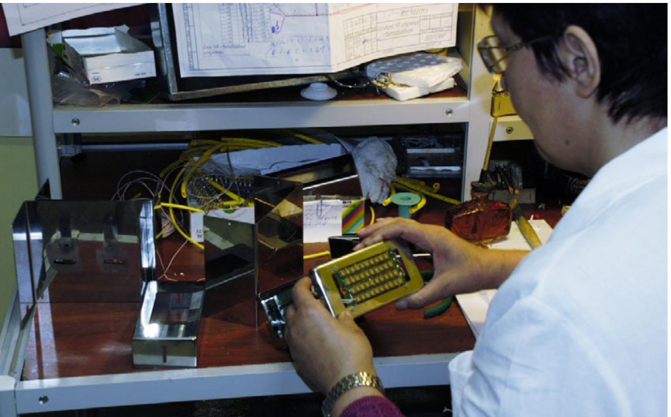
The LED arrays are inserted into the housing in the factory of Sun LLC.
