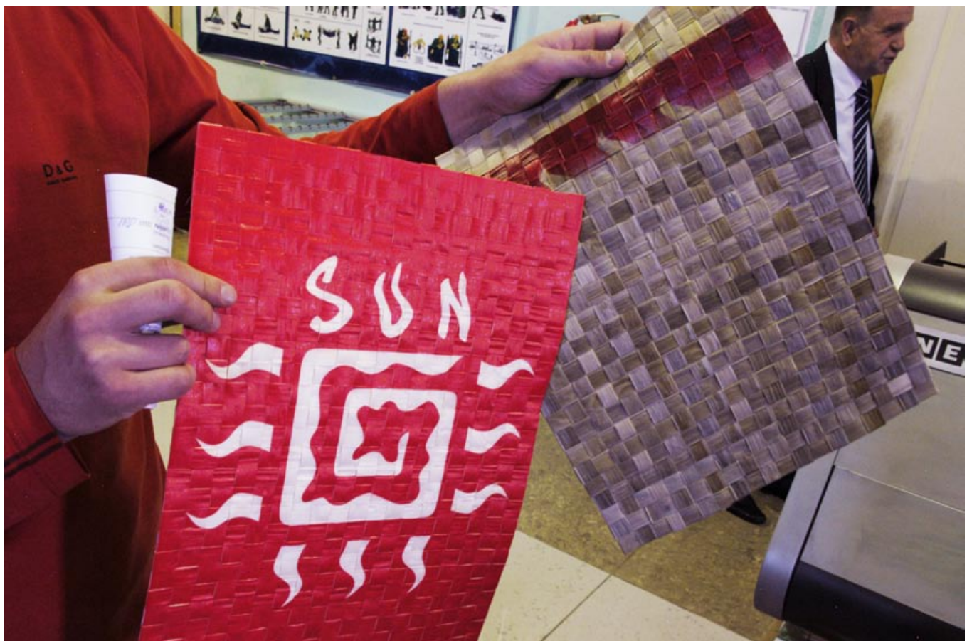
The surface of these wicker table mats were slippery, and this is the one material where the ink will need a pre-coat to better adhere. Otherwise, I did not notice adhesion or scratch problems any worse than with all regular UV ink.
