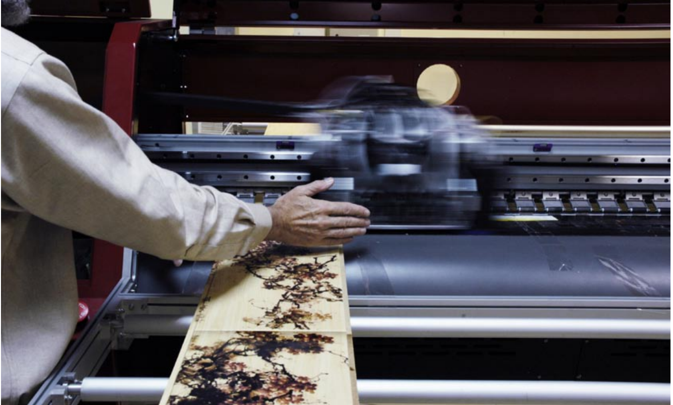
To test if the LED lamps are really not searing hot, I am putting my hand directly next to the lamp while the machine is printing. You would melt the flesh off your hand if this were a mercury arc UV lamp.
