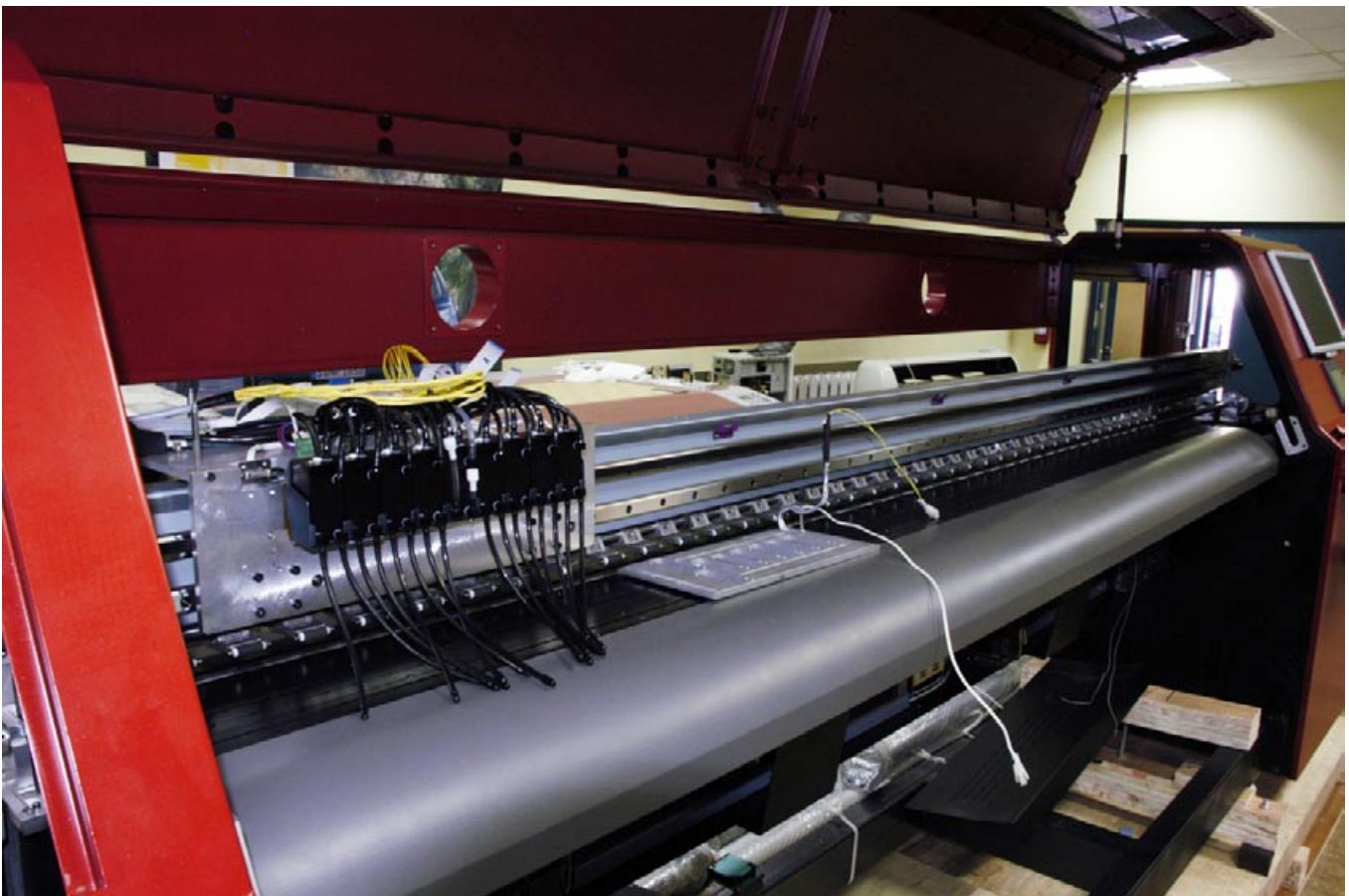
The photo at the bottom shows the recently arrived frame awaiting the insertion of the KonicaMinolta printheads.
