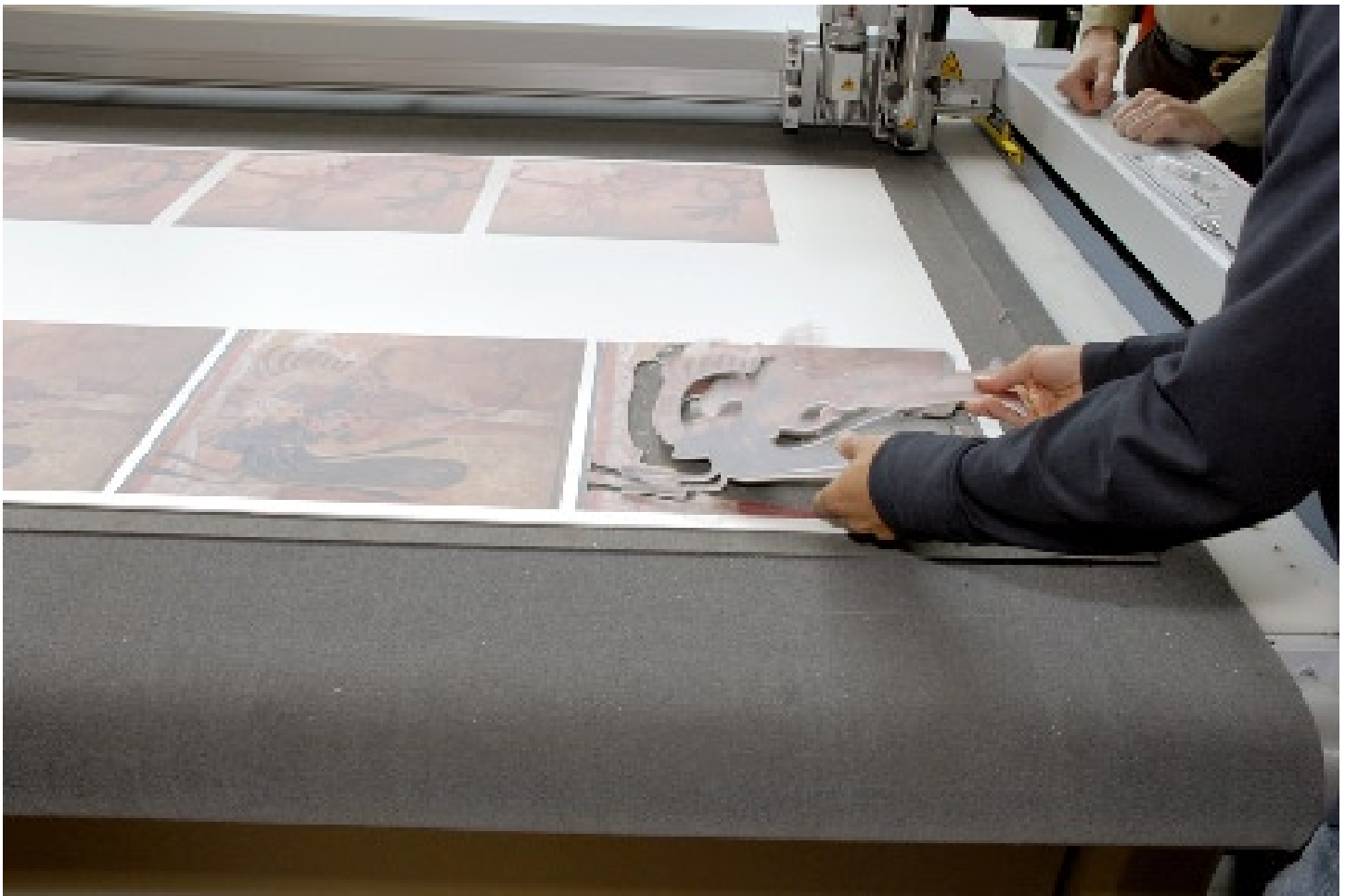
Figure 12. Dibond can also be routed.
