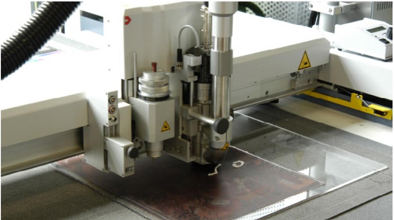
Figure 11a. The toolhead can hold several different kinds of tools, in this image a router bit is used to route a printed plexiglass, the use of this material will be to used as museum displays
