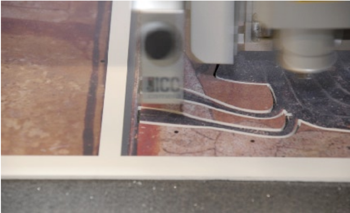
Figure 14. In this image you can see the digital camera of the cutter, in the surface also are registered marks that are followed by the camera to guide the routing head in the routing process
