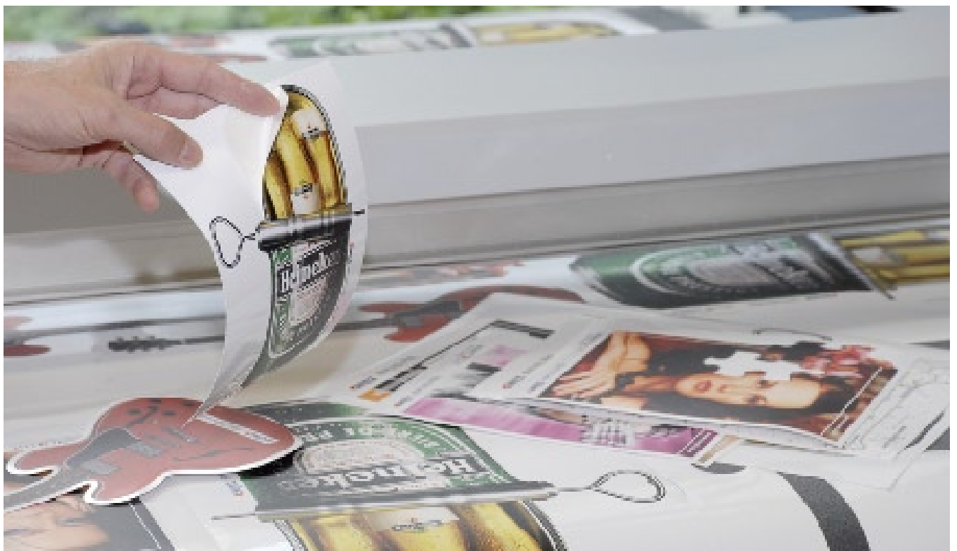
Figure 20a and 20b. Stickers can be thorough cut, and the production process is reduced to programming the cutter and feeding the material.
