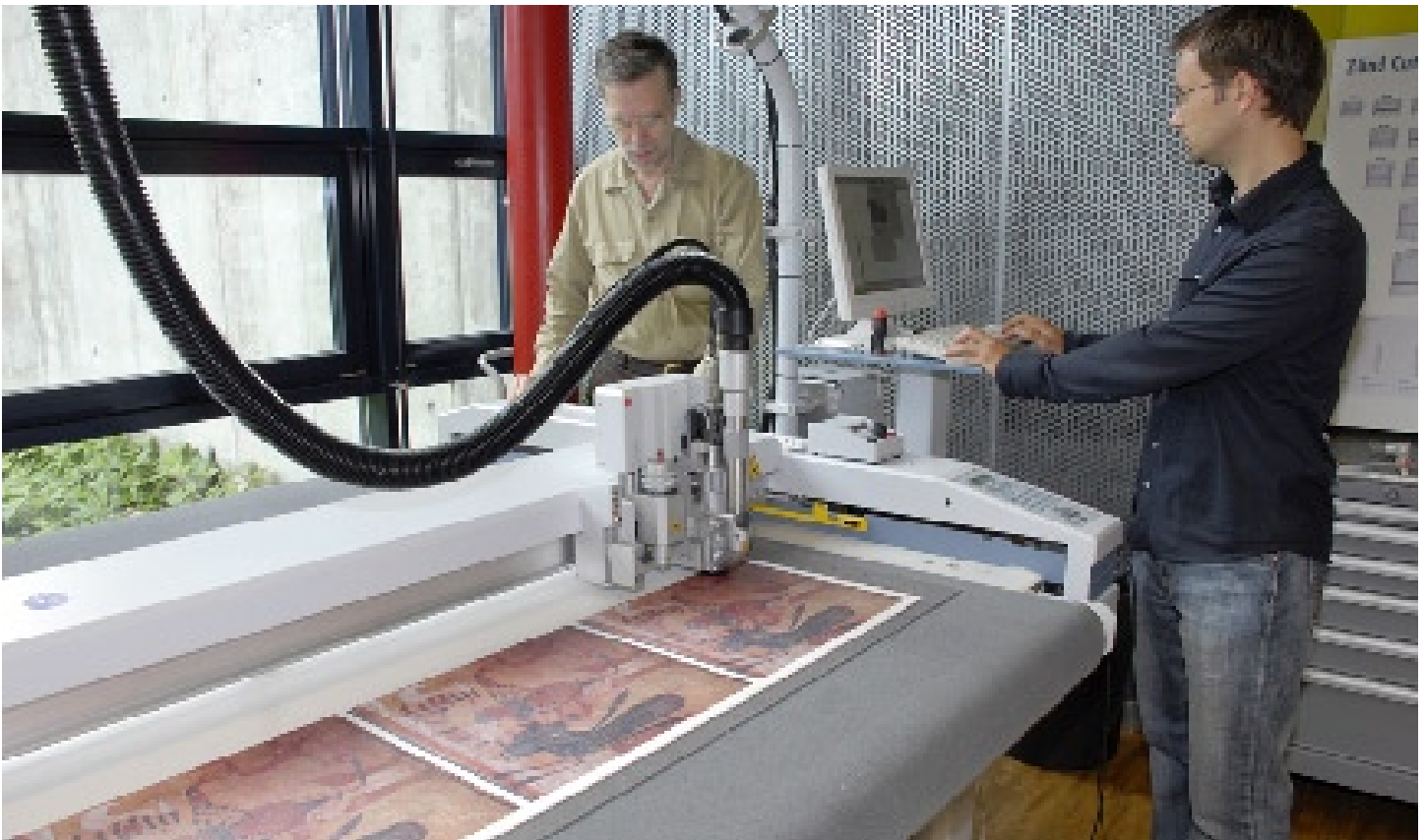
Figure 13. From the computer screen the software is programmed to read the vectorial paths of the file to start the cutting process.
