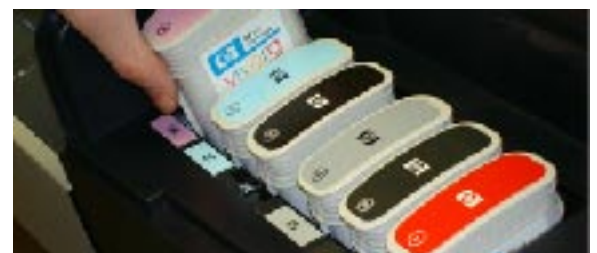
Installing inks in the right panel.
