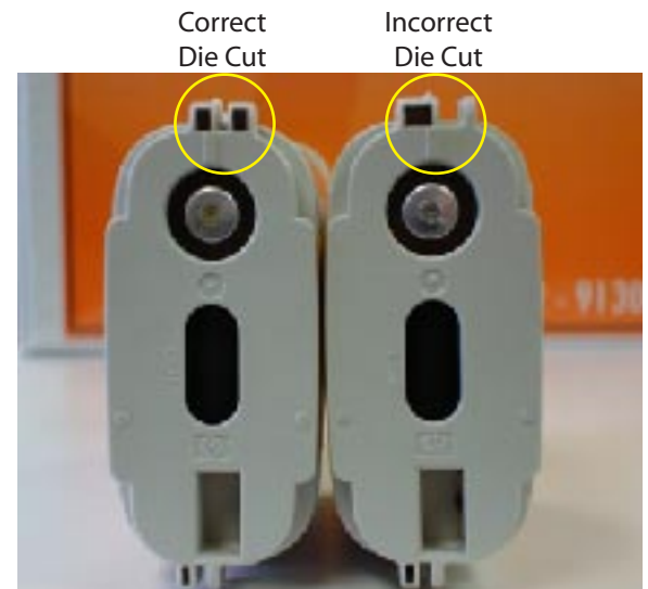
Yellow ink cartridges supplied from Parrot Digigraphic (left) and Hewlett Packard (right).
