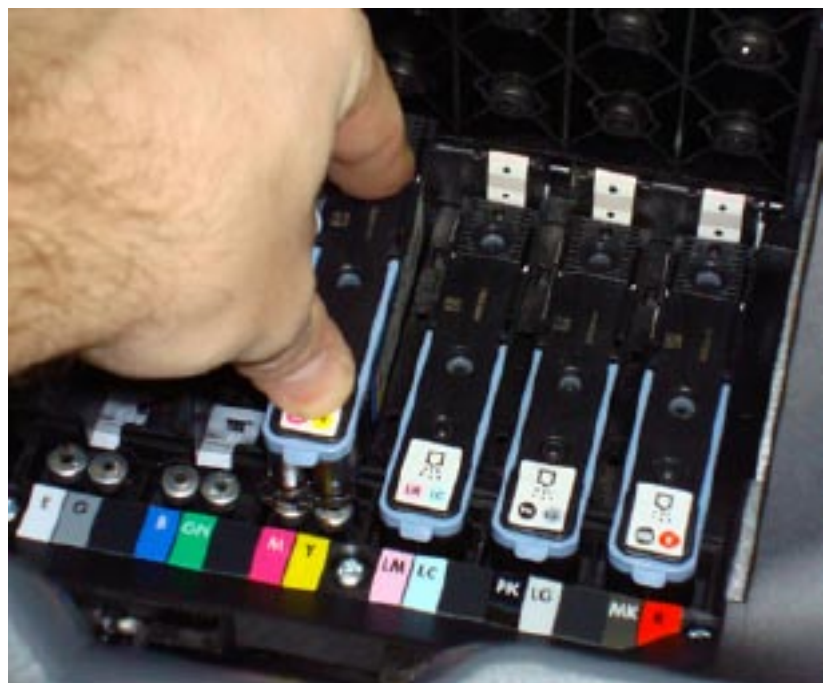
FLAAR personnel places printheads during a printer set-up evaluation at BGSU, Ohio, US.
