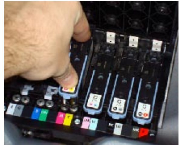
Installing the supplied printheads.
