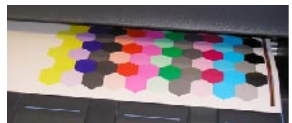
Calibration chart printed when calibrating any specific media.
