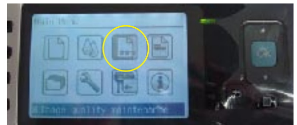
To begin calibration, use the front panel to navigate through the Image Quality Maintenance option.
