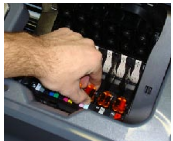
Removing the printhead plugs to install actual supplied printheads.
