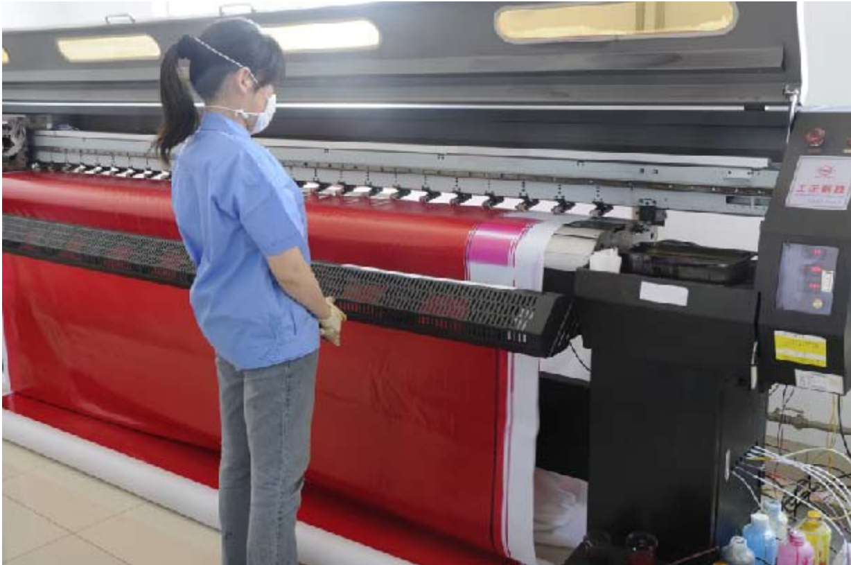
Quality control staff is checking the quality of this batch of ink by printing test of 10 square meters twice, only when the print-work is 100% perfect, the ink can be approved for delivery.
