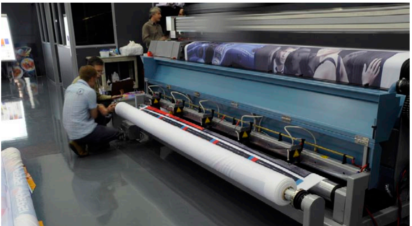
The printer exhibited at Gandinnovations demo room has 5 hot knives.
