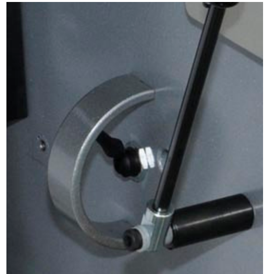
Rear index roller (c) also called stepper roller. The pinch roller (d) is a continuous roller that is lowered and raised with a switch. In the picture at the left you can note that the rear index roller and the pinch roller have different surfaces (the pinch roller has a glossier surface).
