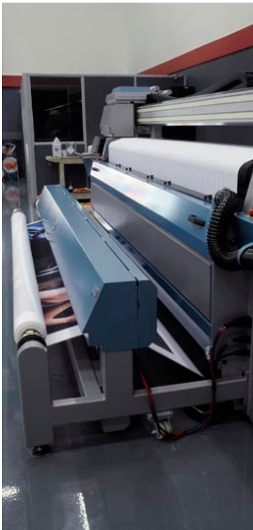
This is the slitting unit that works with heated knives.
