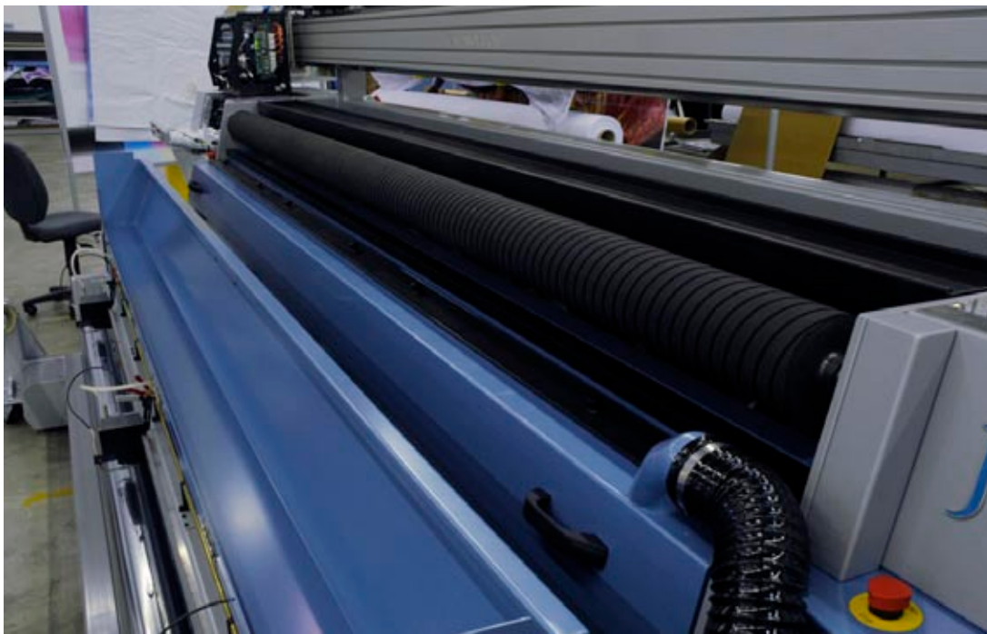
The rollers should be cleaned as well. The printing area has a trough to capture ink. Waste tank should be replaced daily, but this depends on the use.
