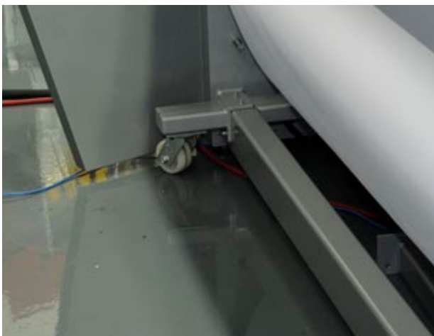
Besides the wheels, the printer has leveling supports in the printer and in the rewind unit.
