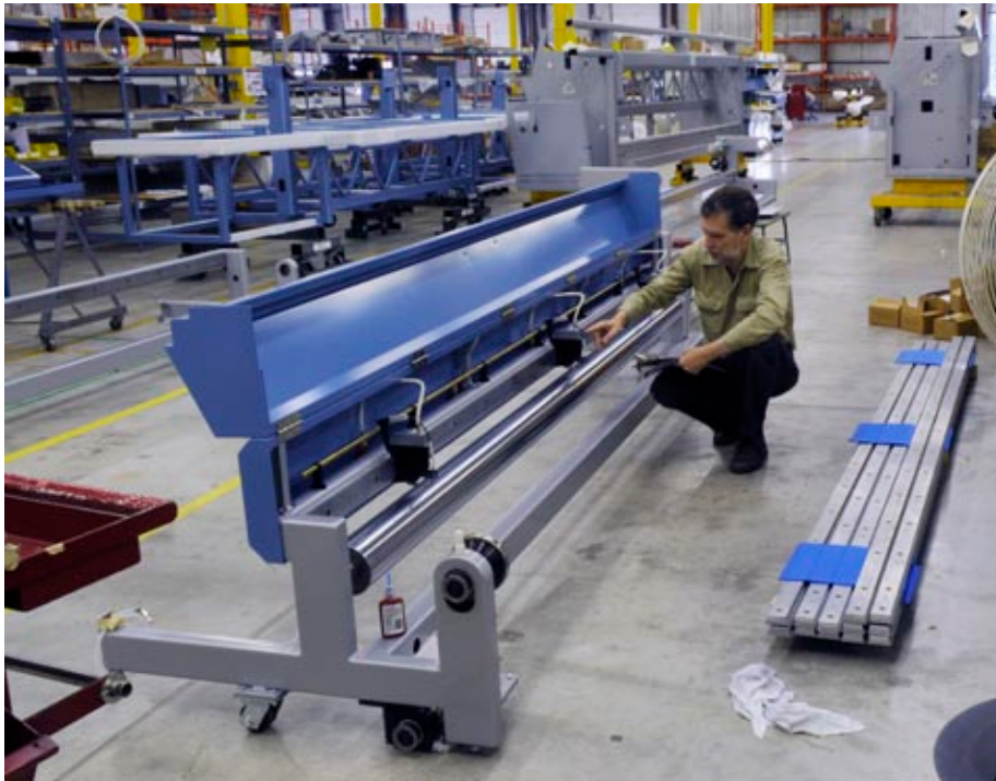
The Jeti 3324 AquaJet has a system of hot knives to cut media once it has been printed on and rolled into the take-up roller. Any operator should be careful not to touch these knives while the printer power is on.
