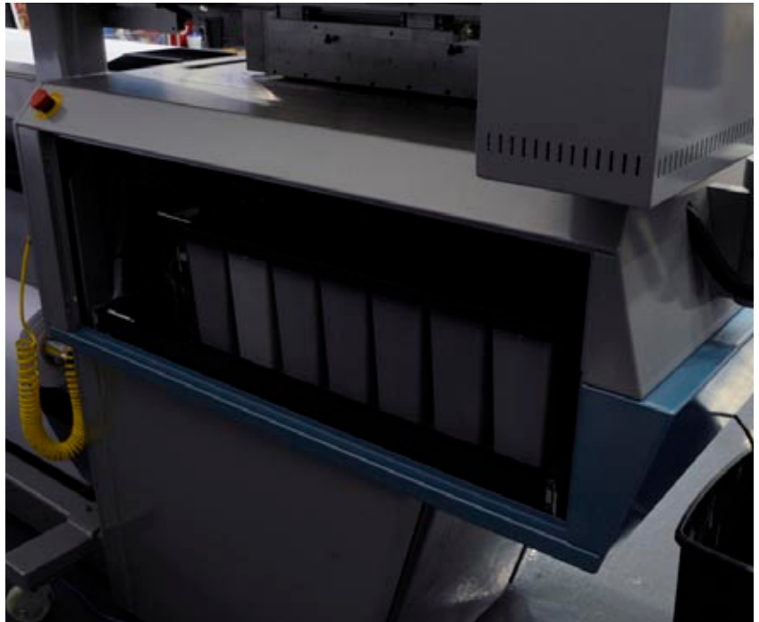
New ink is poured into the printer containers, located at the back of the operation area.
