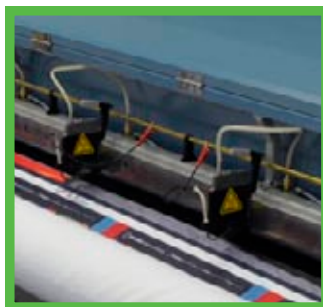
The cutting unit is a system of hot knives
