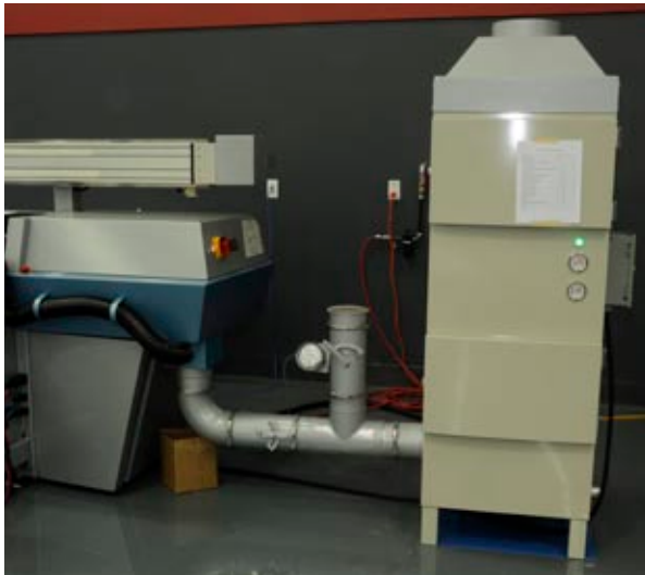
The printer is connected to an exhaust unit through a duct to get rid of aqueous vapor oil and debris.
