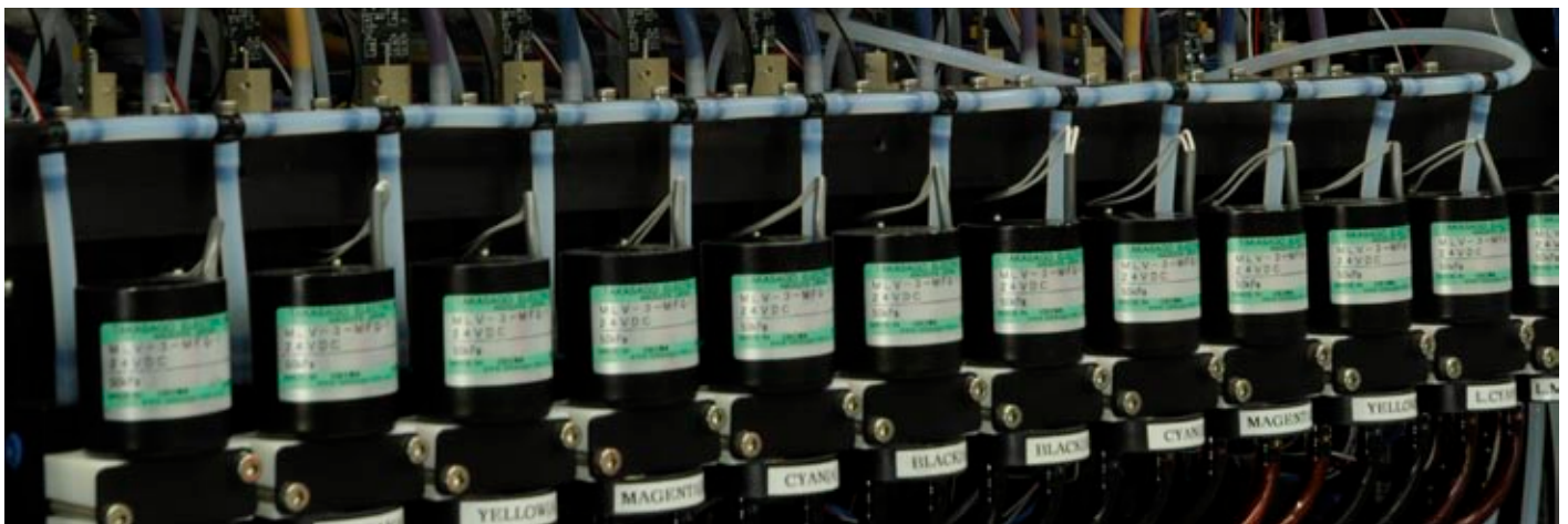
On top of the printheads you can see the secondary ink reservoirs. Ink is heated here before getting to the printheads.
