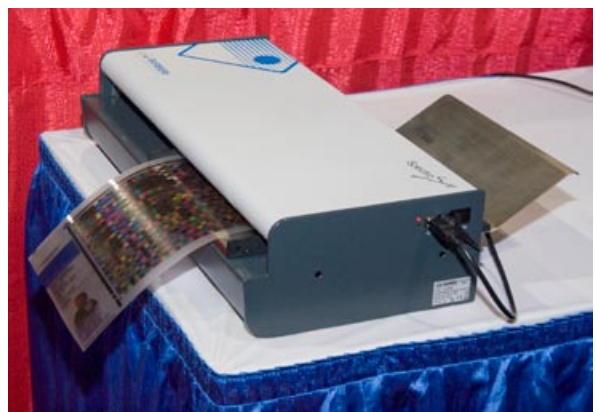
BARBIERI Spectro Swing RT, used for building a color profile (in this picture for transparent backlit media).
