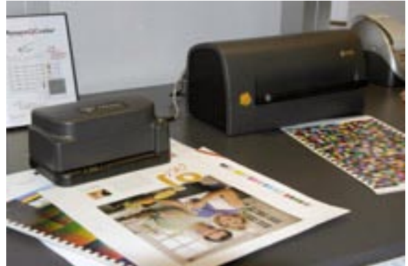
The X-rite and DTP70 are some of the color instruments used in bulding a color profile.
