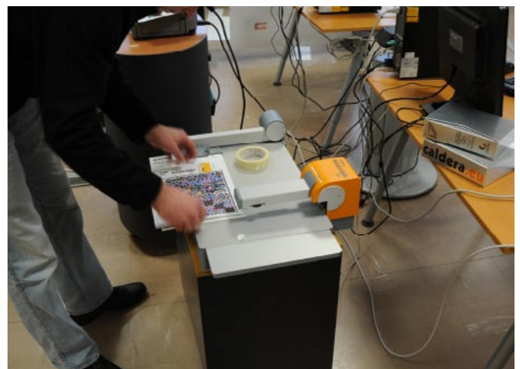
Calibrating the RIP with the spectro profile.
