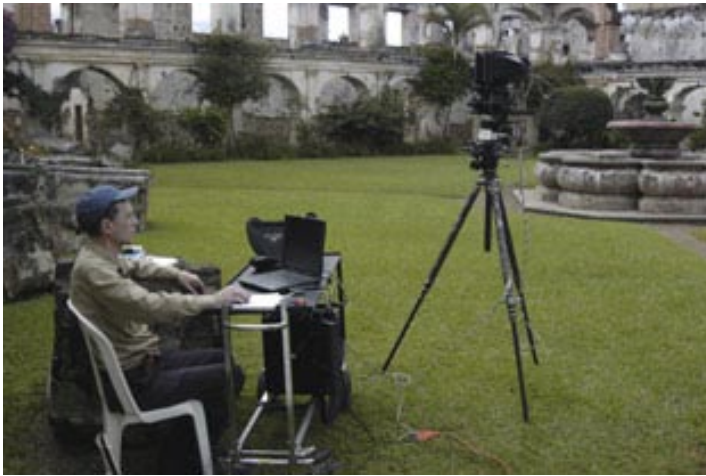
Nicholas doing panoramic photography in 17th century ruins of Spanish colonial church in Antigua Guatemala. The equipment consists of Gitzo Tele Studex tripod, Manfrotto tripod head, BetterLight Pano/WideView motor, Cambo Ultima 4x5 camera, Schneider lens, and BetterLight Super 6K tri-linear scanning back.
