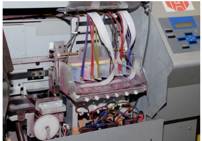
The printhead cleaning area is easily accessible once you remove the hood. But to remove the hood (not shown here) requires taking off two screws.
