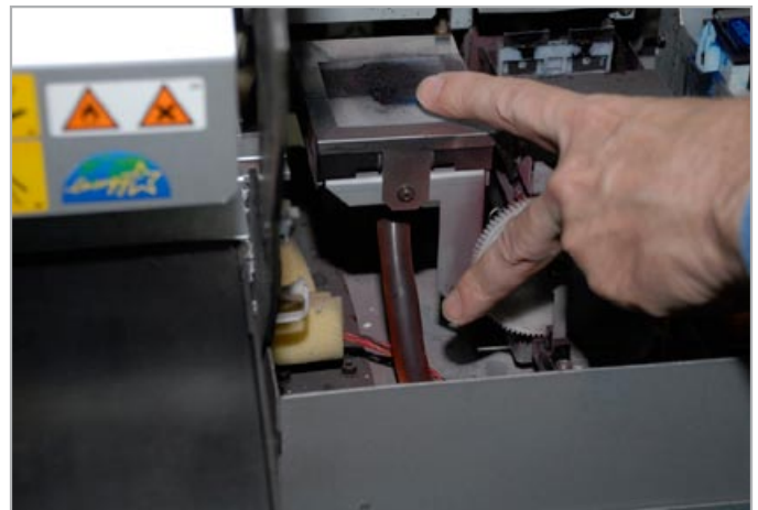
The spitting gutter is the white pad that receives the ink the print-head spits and leads it through a tube into a waste bottle.
