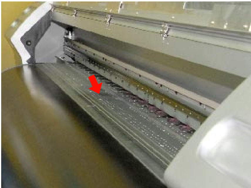
A Suction fan holds media flat through these area of holes.
