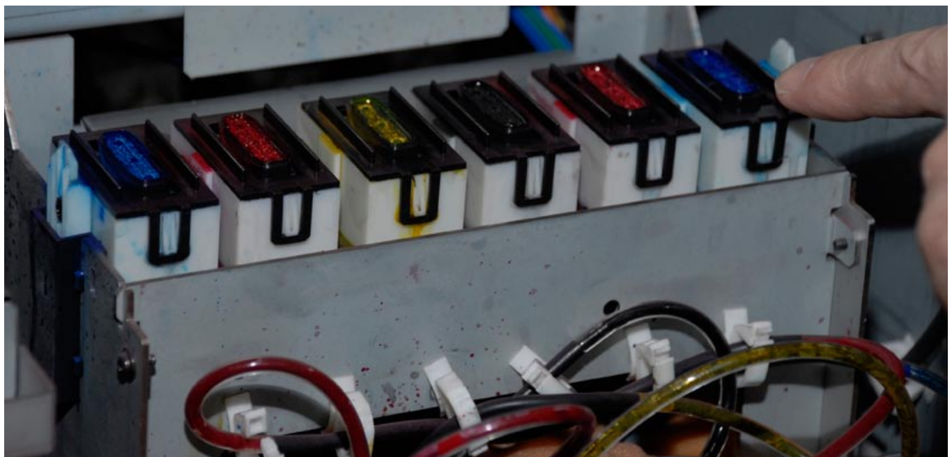
Printheads are in a single row; you can see this in the positions of the capping stations
