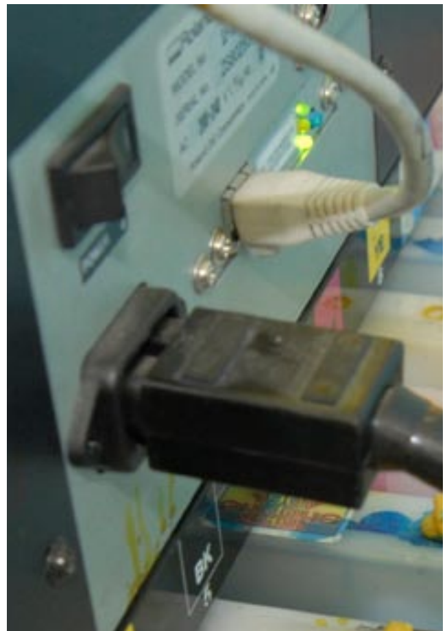
Ethernet connection. AC 200-240 voltage is required
