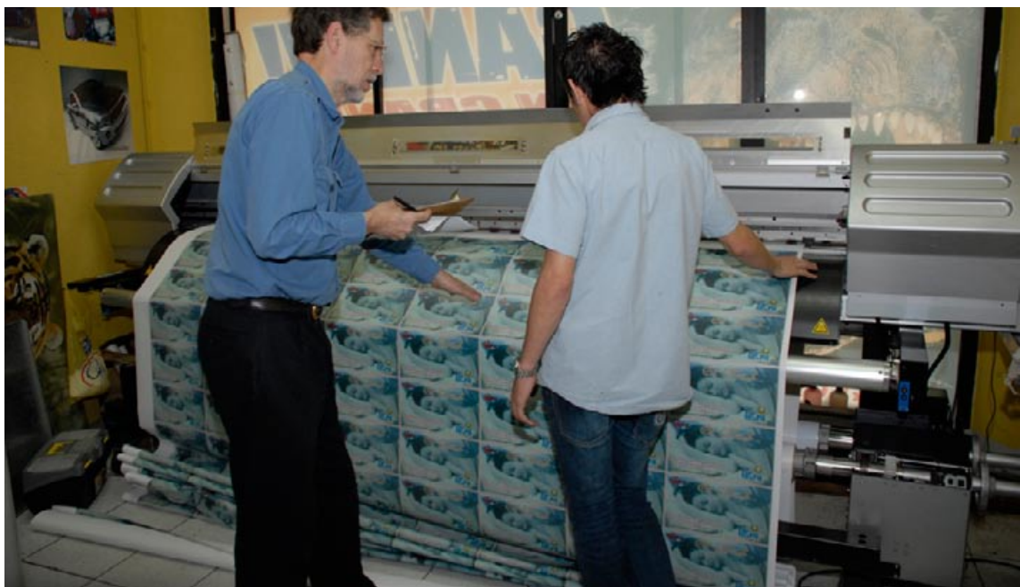
Media is fed from bottom up into the printer
