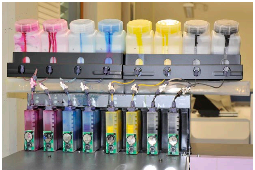
Sepiax inks being tested with a Mimaki printer.
