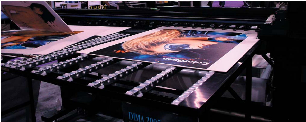
ColorSpan 72 UVR UV-cured flatbed printer.
