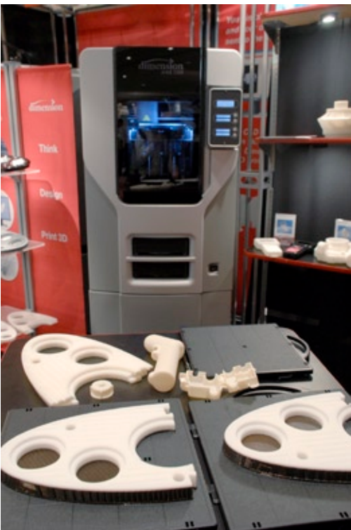
Dimension 3D RP machine and samples.
