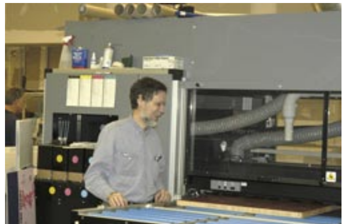
Durst Rho 160 at SFC Graphics, Toledo, Ohio. If you need any material, thick or thin, printed upon, SFC can handle it with this sophisticated UV-curable ink flatbed printer.
