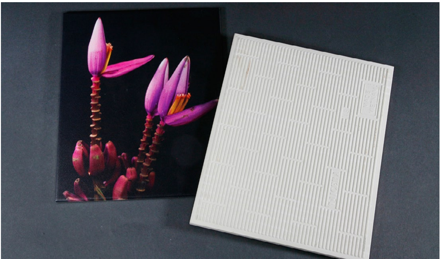
These are the most beautiful ceramic tiles I have ever seen printed on any UV-cured flatbed printer. The color gamut is superior to most others and the image did not scratch off. You can license the primer and obtain this from GCC, contact sophie.chang@gcc.com.tw to inquire about this primer.
