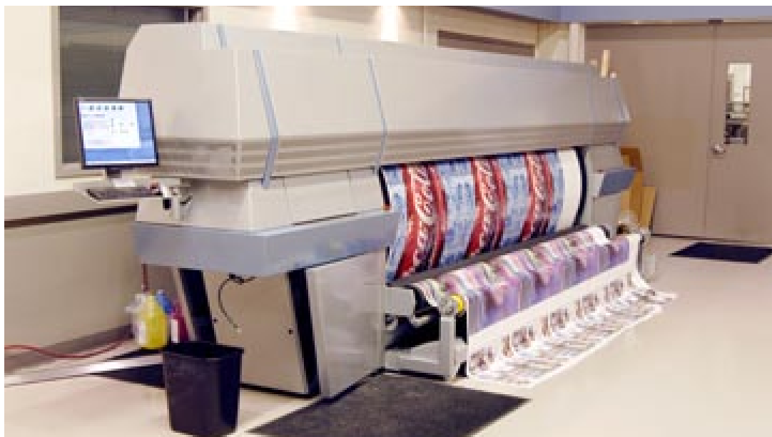
This is the new enclosed version of the Gandinnovations Jeti 3.3 solvent ink printer. Enclosures help with air quality control, especially in countries or states such as California that have stricter rules than other places
