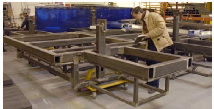
Inspecting the core structure of a Gandinnovations Jeti flatbed inside their factory in Canada
