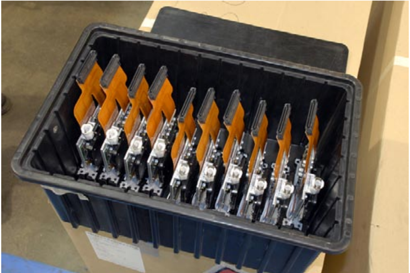
VUTEk printheads as they arrive to be added to the printer in the factory
