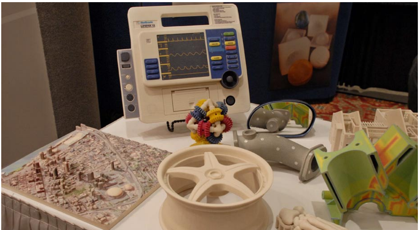
ZCorporation models at RAPID 07. Plaster-like powder is the main substance used in the ZCorp printer
