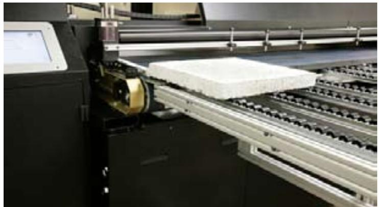
*ColorSpan 9840uv printing on concrete*
