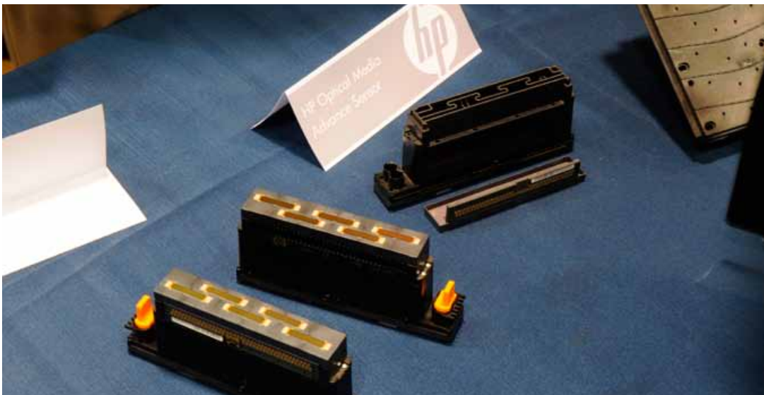
Wide area HP printhead modules, a new trend that allows faster printing for serious production.
