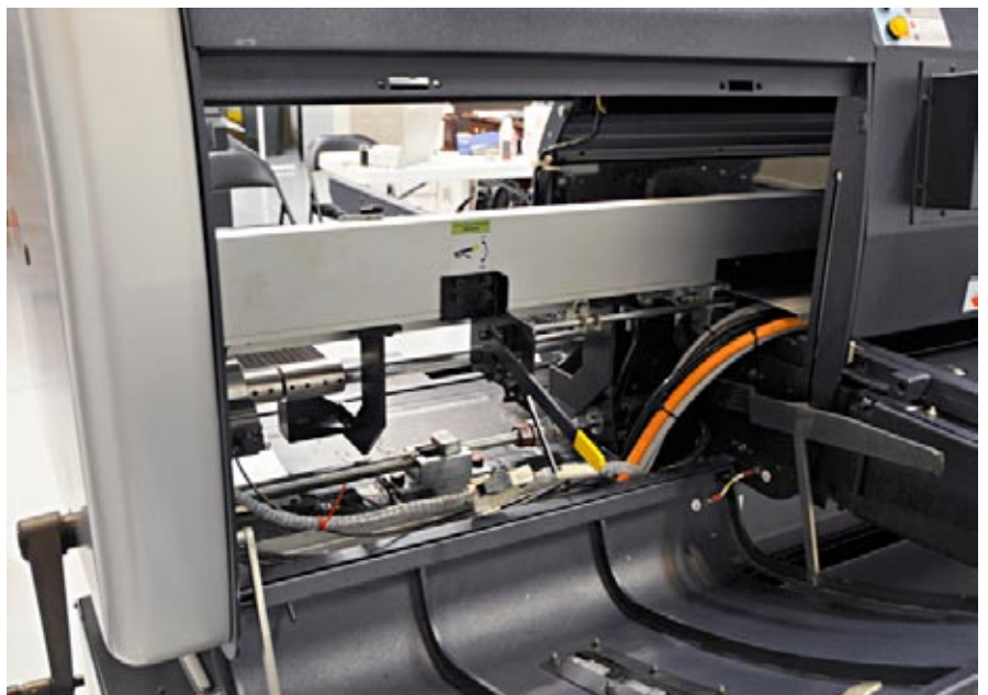
Service station, located at the right back of the printer.
