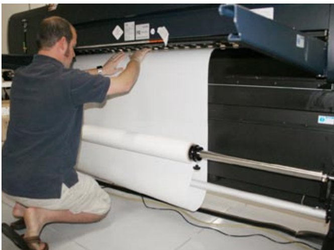
Loading and preparing the roll-fed media for printing.
