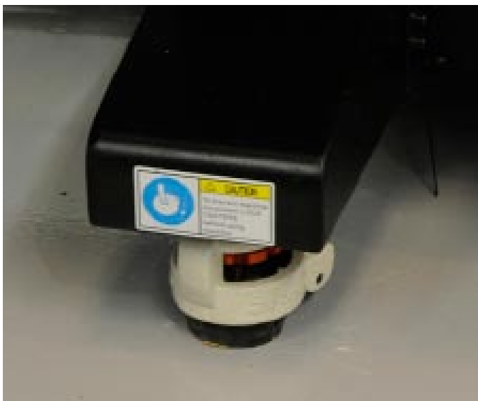
The printer has wheels and leveling supports built in the same structure.
