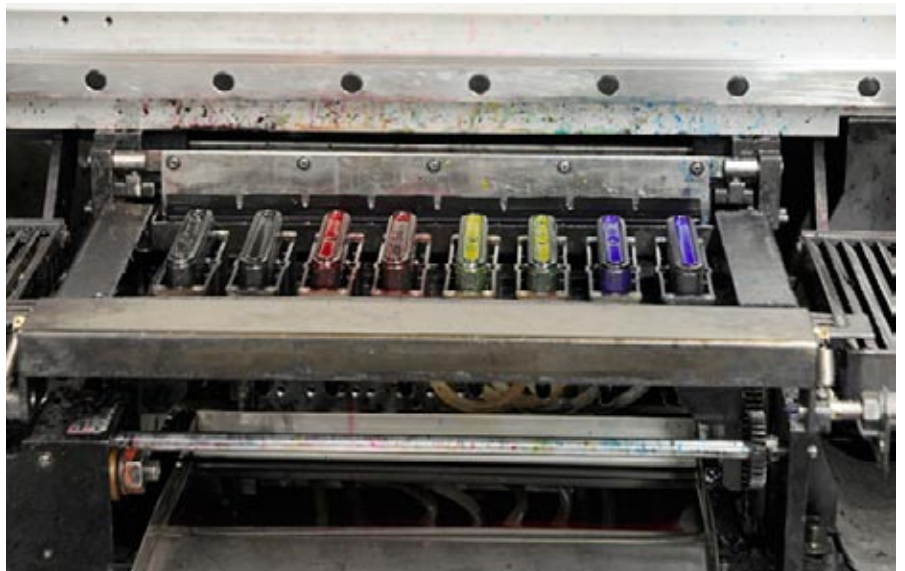
Printhead capping station
