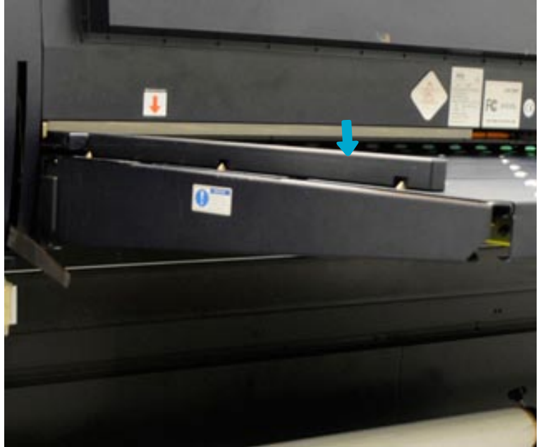
Alignment bar at the rear table.
