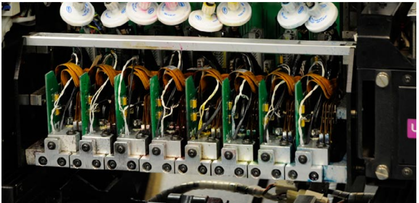
The printheads are located in a straight row.
