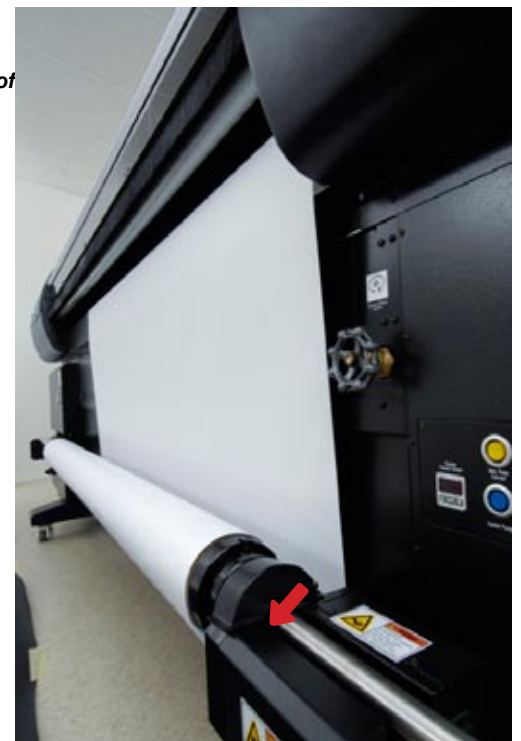
Take-up roller. Roll-fed media is held in a spindle at the back.
