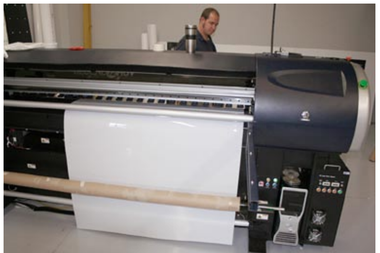
Loading and preparing the roll-fed media for printing.
