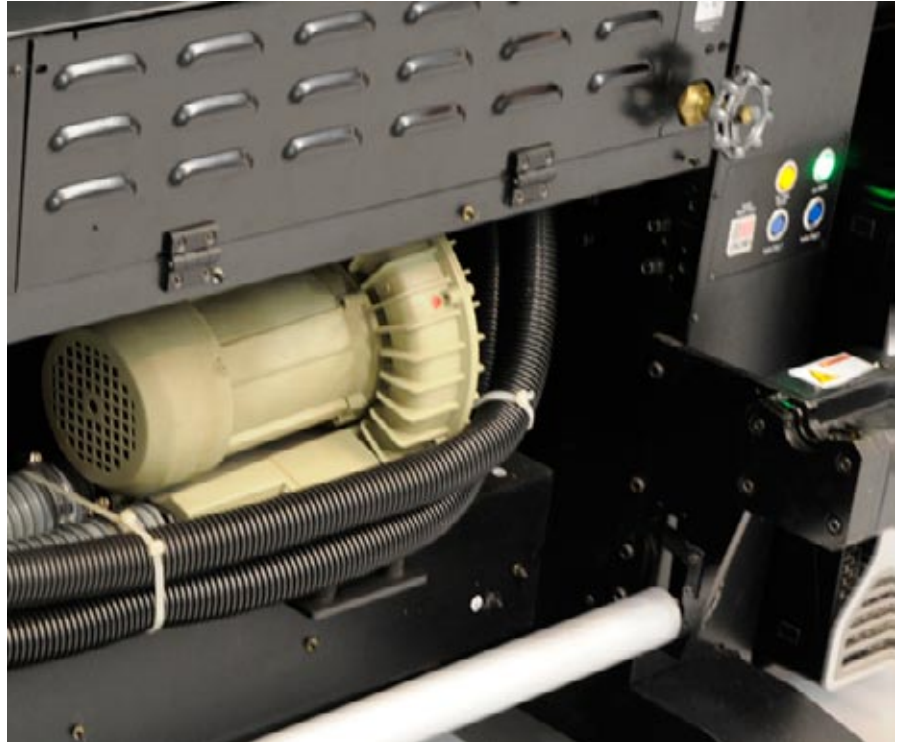
The vacuum area is created by two pumps. In the picture below, you can see the vacuum control buttons. The vacuum areas are user-definable.
