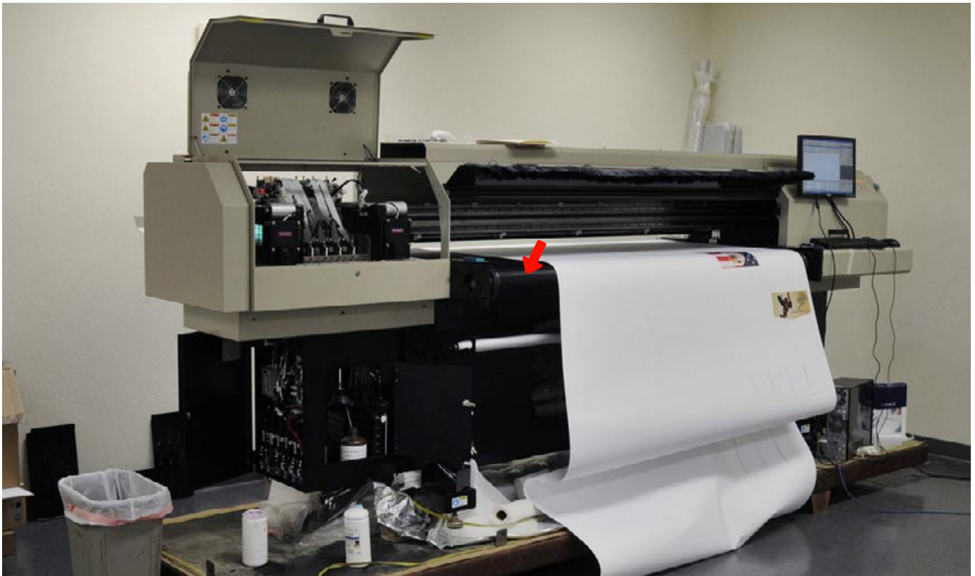
The machine has a transport belt; FLAAR clasifies the H700UV as a Combo Printer.
