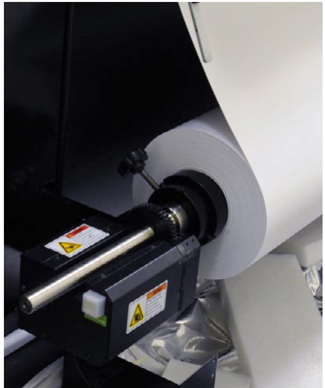
The roll is held on a spindle.
