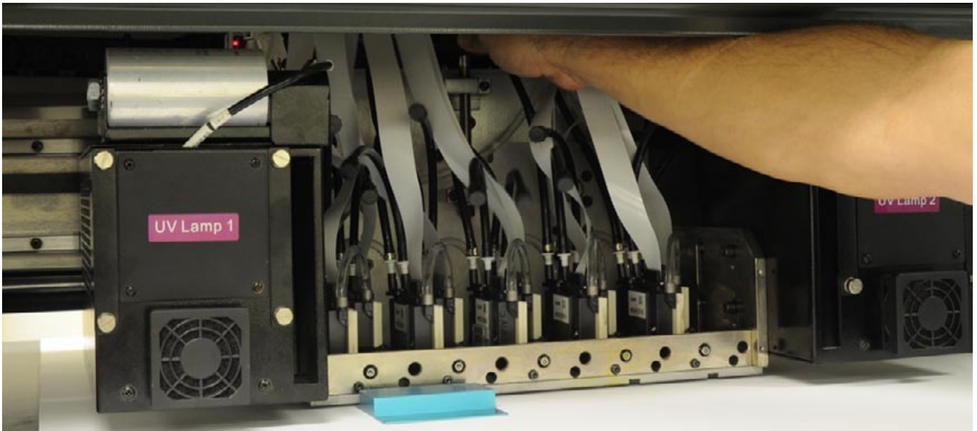
The printhead carriage height is changed manually.
