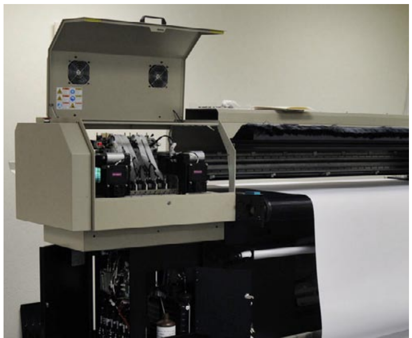
Cleaning station can be easily accessed. It is at the left.
