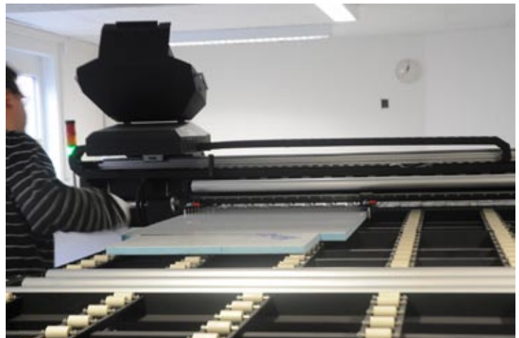
Notice the extra piece of material taped onto the end. This extra piece allows the grit roller and pinch rollers to move the board all the way through the platen system.
