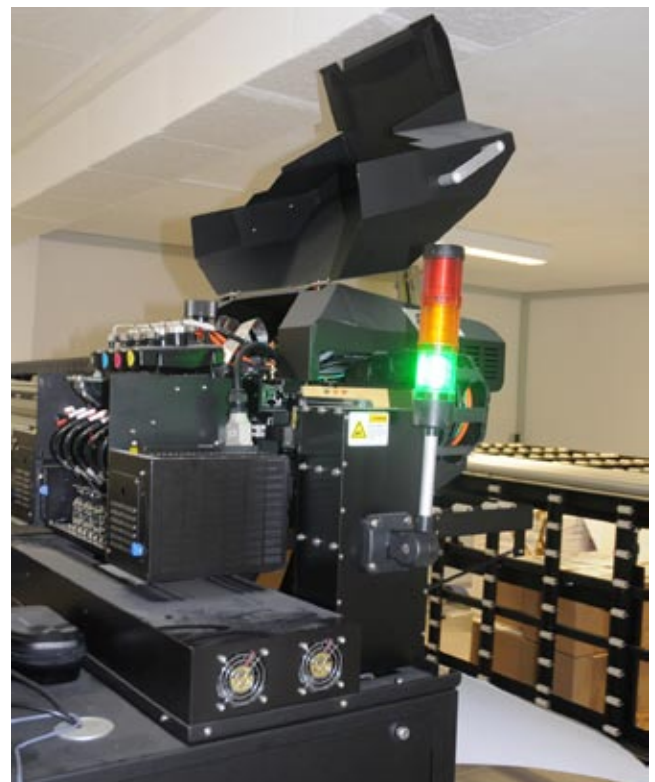
Here you can see the beacon tower of lights, and the two fans at the right end of the printer (to exhaust the heat sink). Notice all the dust that has settled on the printer; this is from the adjacent offset presses.
