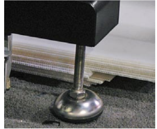
Leveling support of the printer
