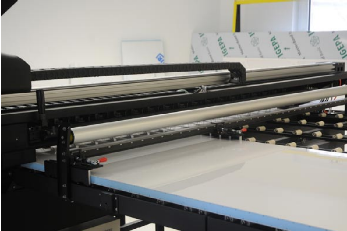
Alignment is at the back left. Other printers align at the back right. There is no one way that is better or worse. Here it makes more sense to align at the same side as the LCD monitor on the other side.
