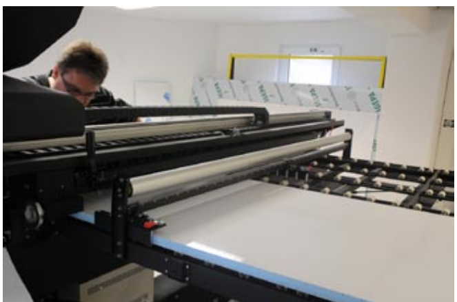
Next step after aligning the sides at feeding area, is to align the front of the board (at the front of the platen).
