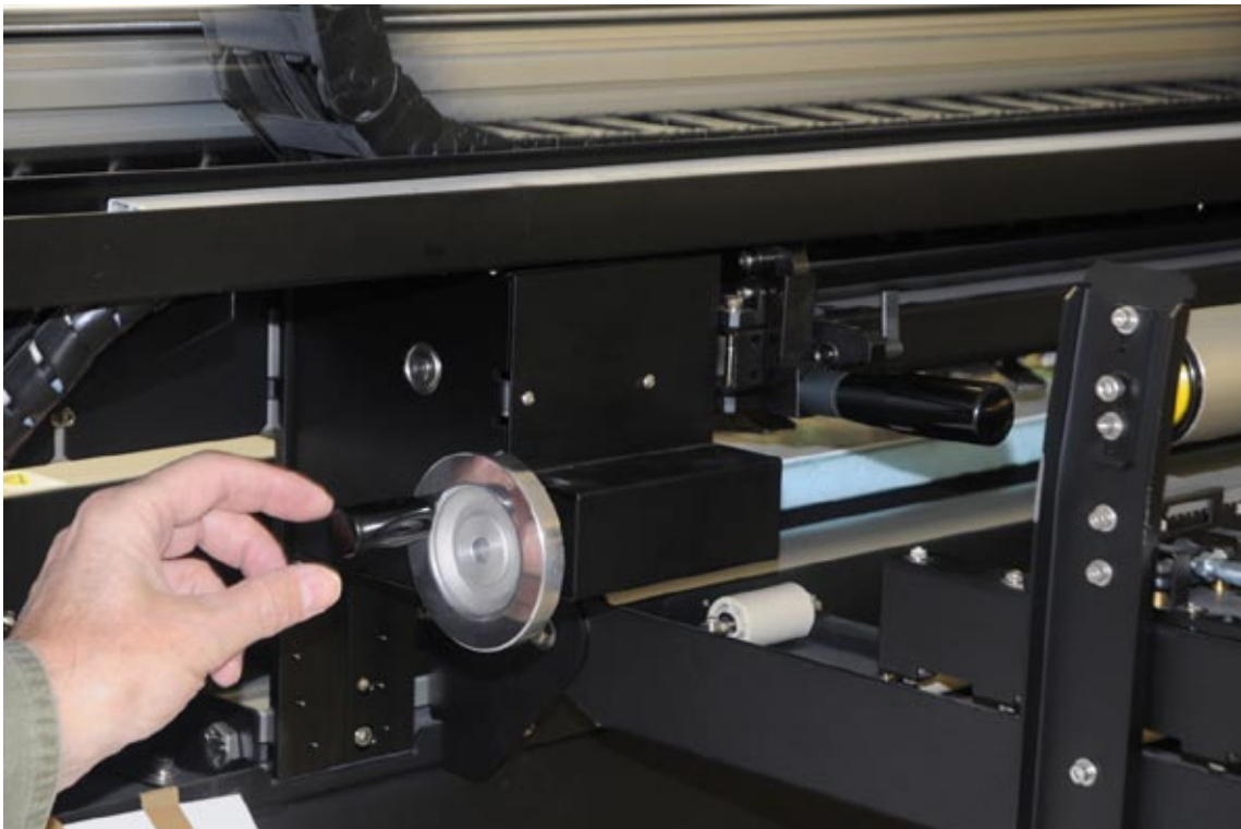
Here is the hand crank to raise or lower the pressure on the pinch rollers.
