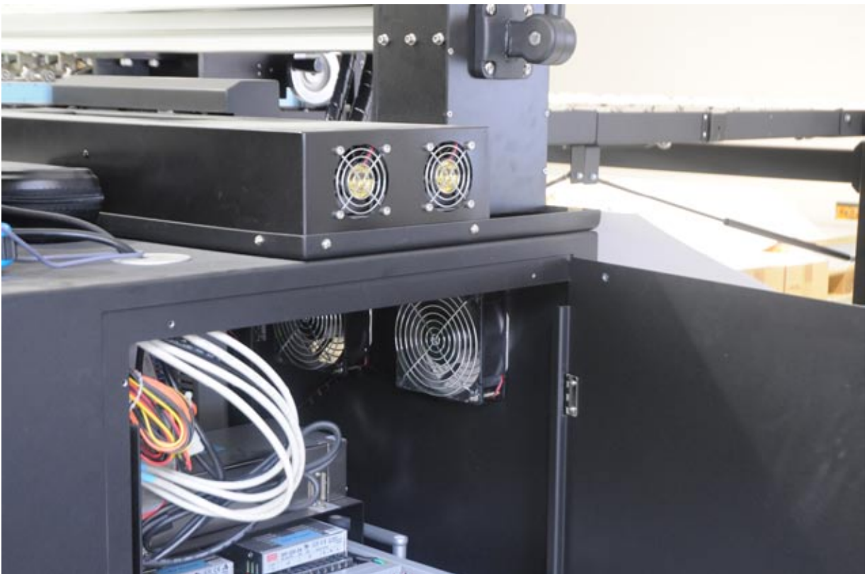
Here you see that the top end fans exhaust from under the heat sink. The larger lower fans exhaust out of the electronics cabinet.
