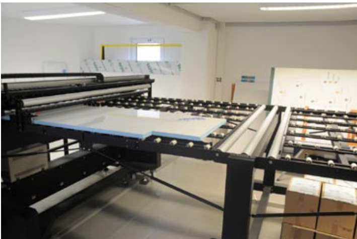
Notice the extra piece of material taped onto the end. This extra piece allows the grit roller and pinch rollers to move the board all the way through the platen system.
