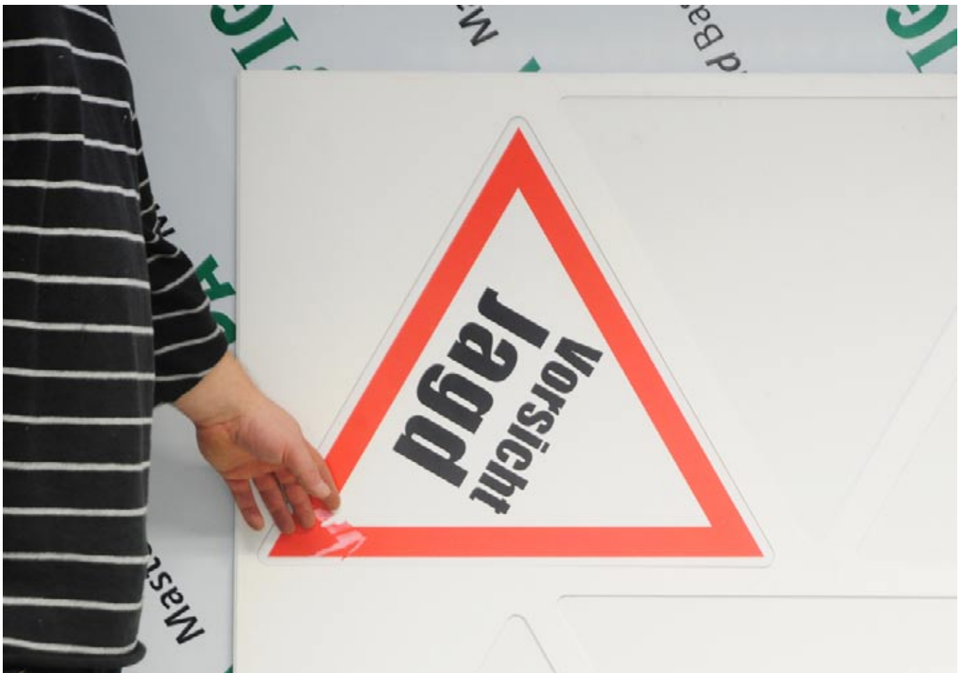
Here is a triangular jig, a custom-cut holder to hold and help guide a triangular object through the printer. This printshop intends to print on a diverse range of materials, much more than just foam-core.
