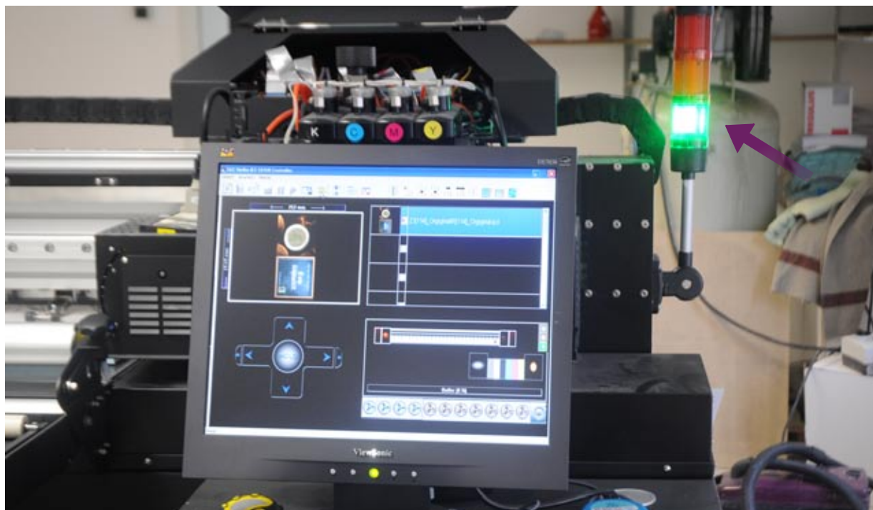
Beacon tower of lights. Not many printers have this system available.
