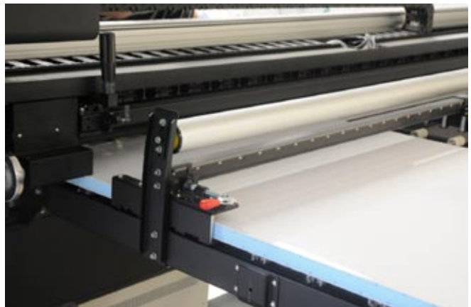
First step is to align the thick rigid material at the back.
