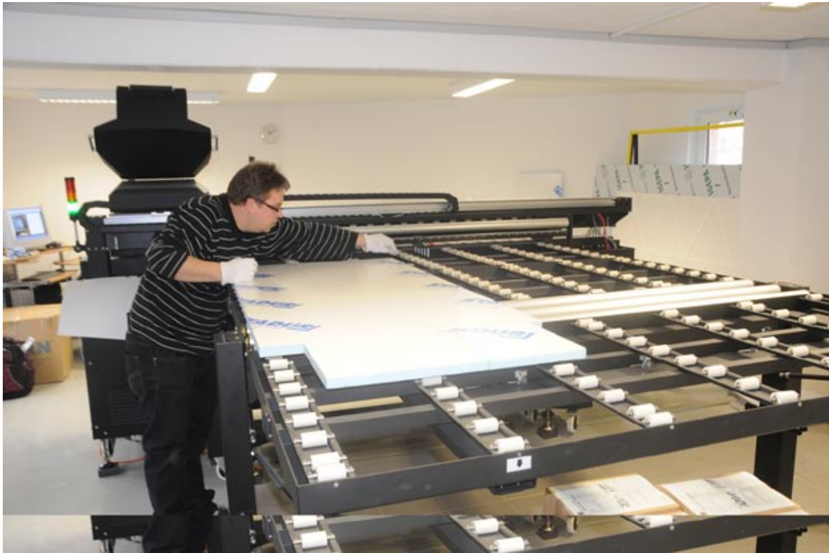
It is essential to wear gloves when you handle boards being printed on with inkjet inks.
