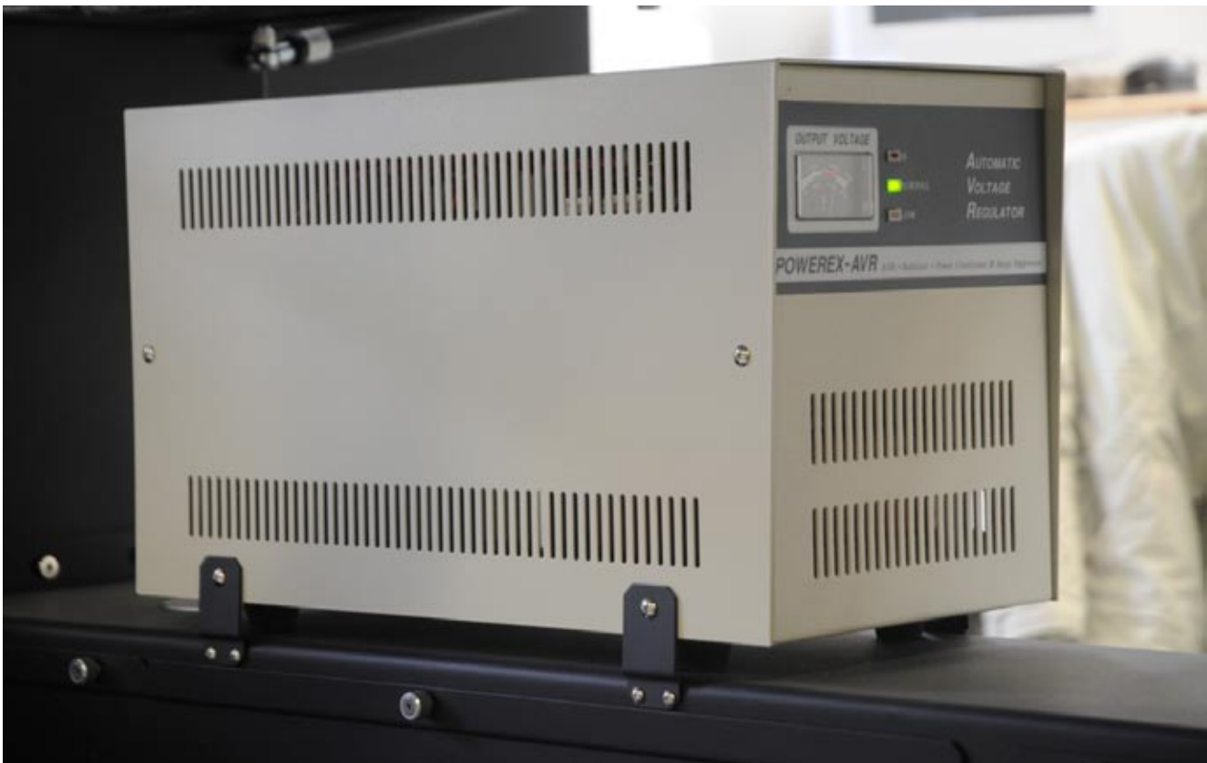
Under the middle of the printer frame you see the Powerex-AVR, a crucial device for protecting the electronics inside your printer. This kind of power line conditioner and protective system is totally missing on most printers that cost under $200,000.
