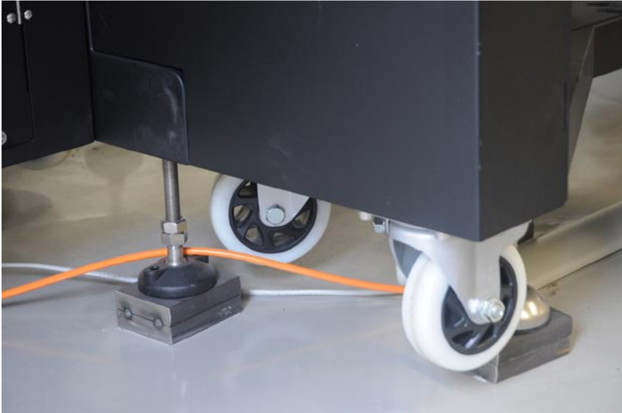
You do not need the wheels once the printer is leveled on the leveling system.
