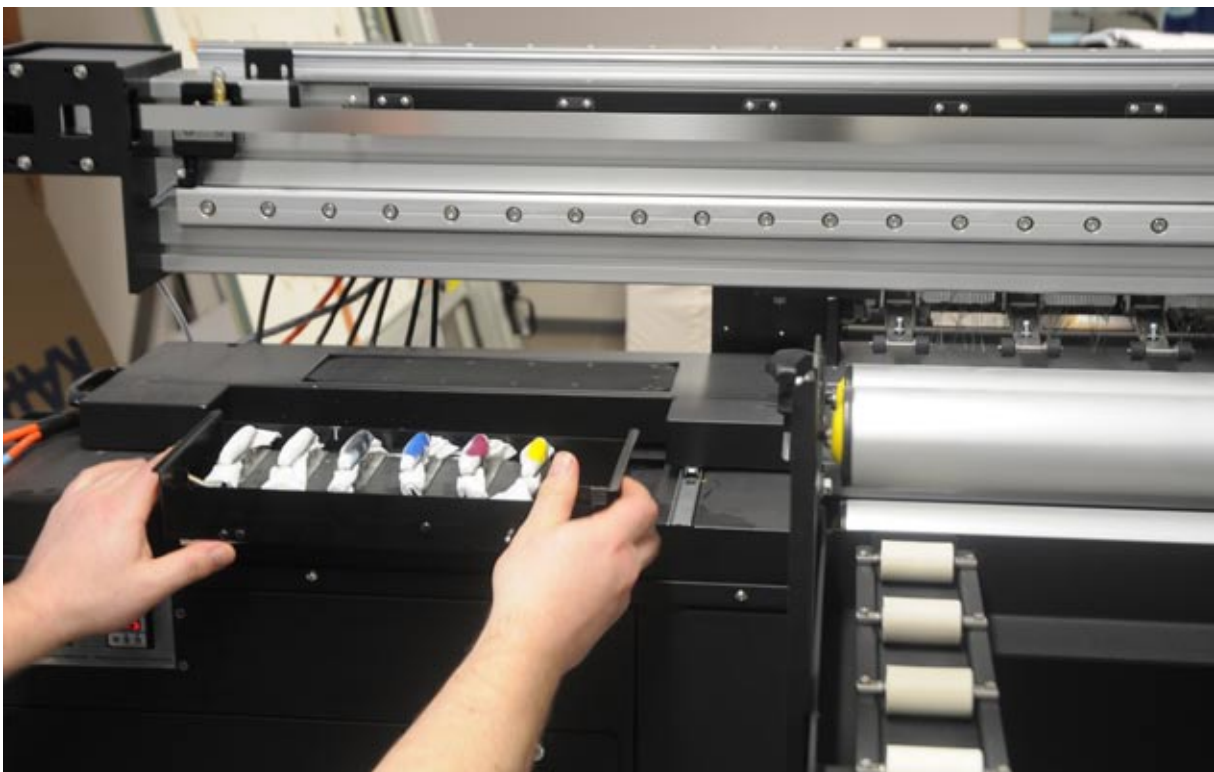
To clean the printheads is very simple. I definitely like how GCC has cleverly arranged this. There is a pre-set “wipe” for each printhead. You use your thumb to wiggle each wipe.
