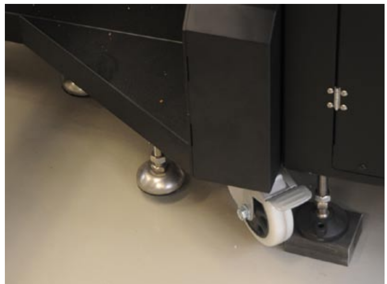
The roll-to-roll accessory has its own wheels and leveling devices.
