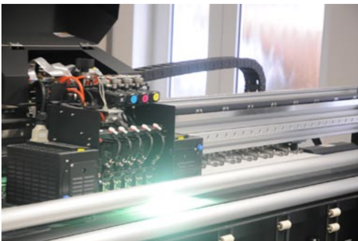
Light leak is high because there is no skirt (or at least I did not notice one). Notice that the hood is raised; this is typical. In all printshops that I visit, they almost always have the hood raised.
