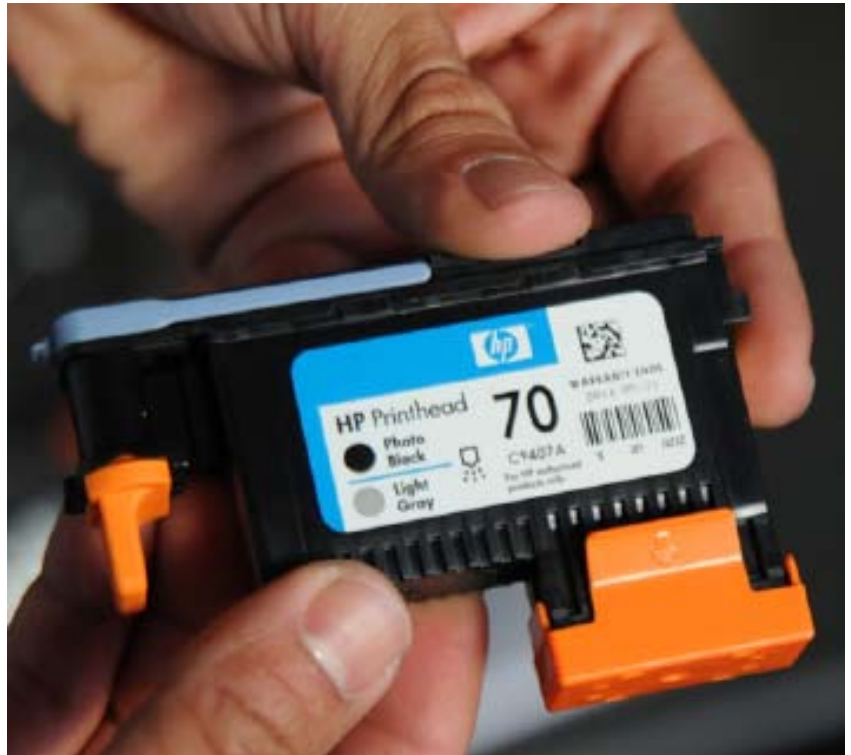
Each printhead handles two colors.
