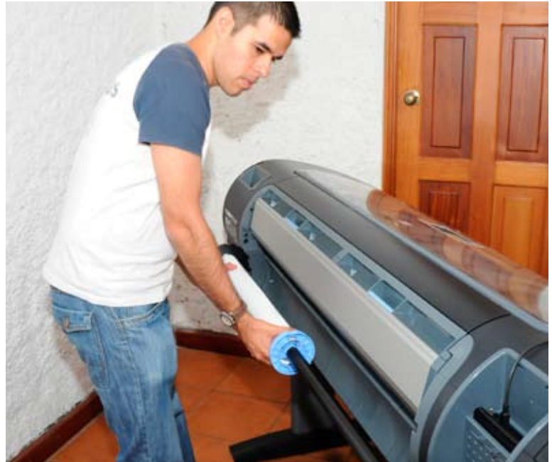
Media is loaded at the back. The instructions to properly load the roll of media were not very clear in the sense that the manual mentions lefts and rights, but it is hard to know if they mean viewed from the back or from the front.
