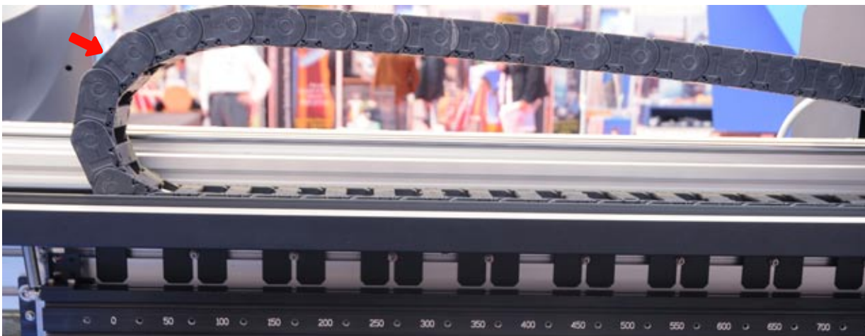
The e-chain is designed with a smooth interior to extend the life of the cables. The links provide flexibility without pressing or bending cables.
