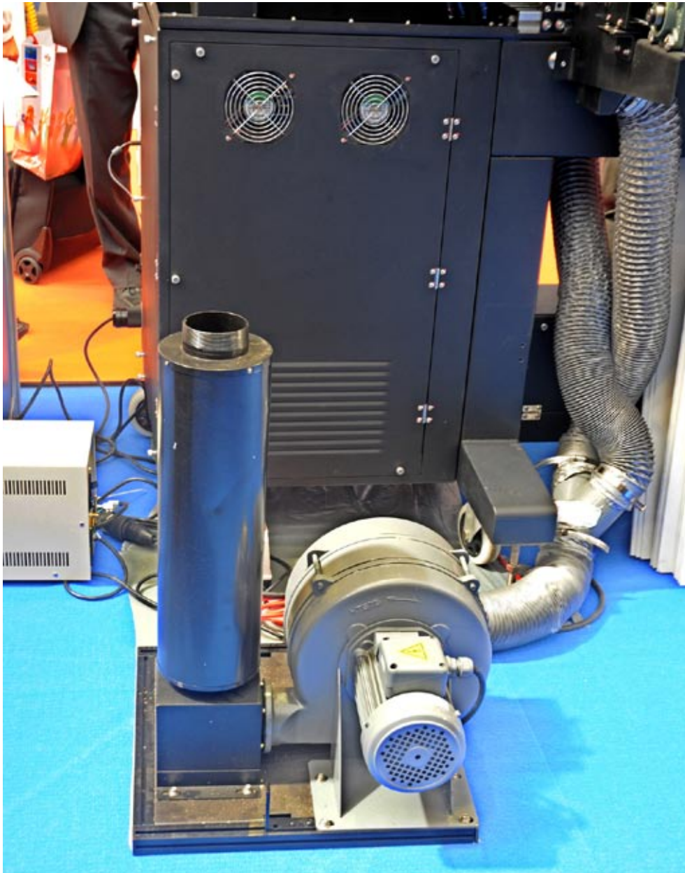
Vacuum is created by this air pump. As you can see, the main hose divides in two hoses for the vacuum areas.
