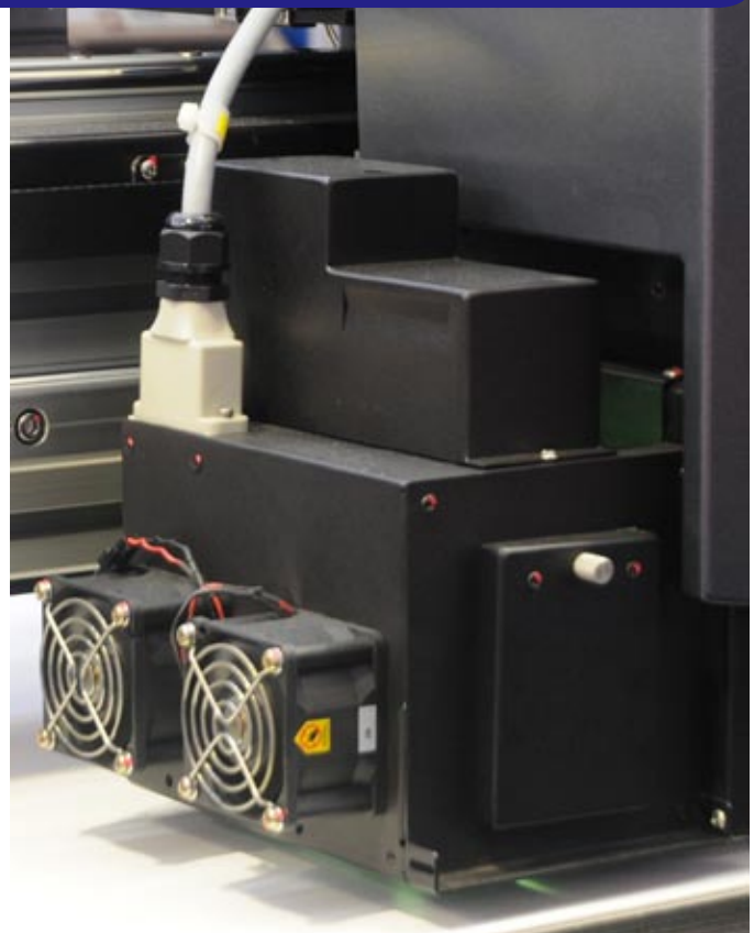
The UV lamps are cooled by two fans at the side of each lamp.
