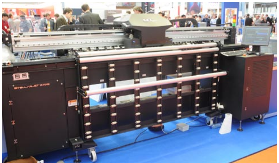
GCC StellarJET 183UVK hybrid printer. The K72UV is an upgraded version of this printer. The main difference is that the 183UVK moves media with pinch rollers (hybrid mechanism), whereas the K72UV moves media with a transport belt (combo mechanism).
