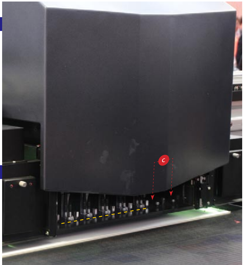
We drew an imaginary yellow line to show that the printheads are placed in a row. At the right end of the space for printheads you see two empty slots (c) for the optional colors.
