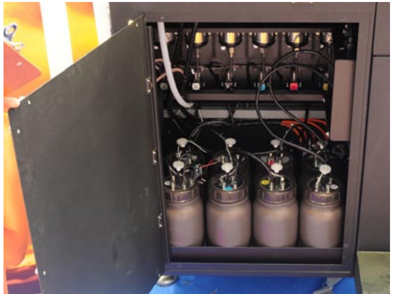
Ink containers are located in the left cabinet. As you can see, all the containers and tubes are dark to avoid exposure of ink to sunlight.
