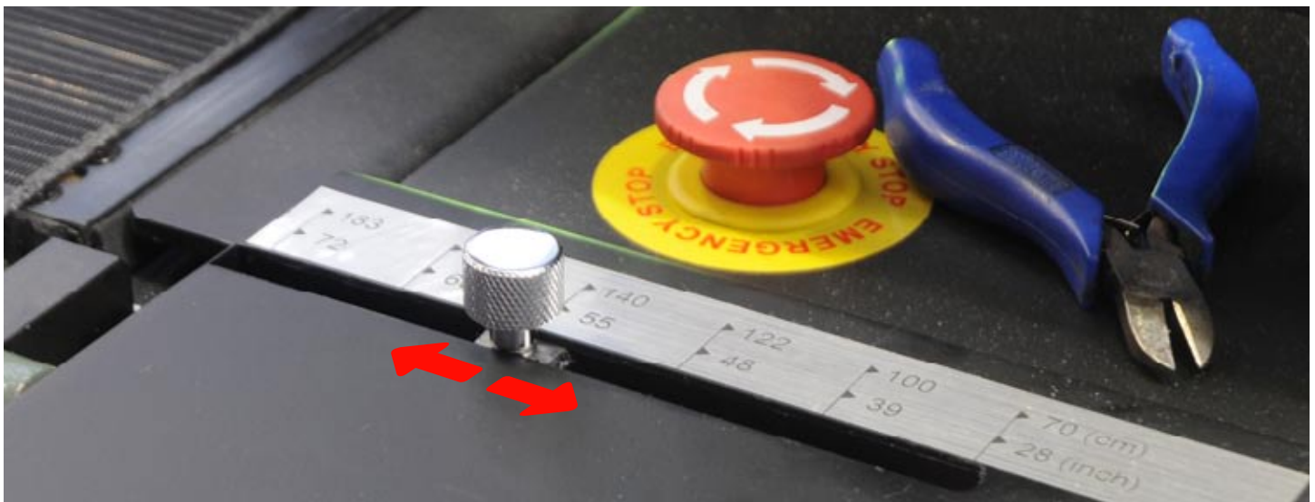
This is the manual slider to turn on/off the areas of vacuum.
