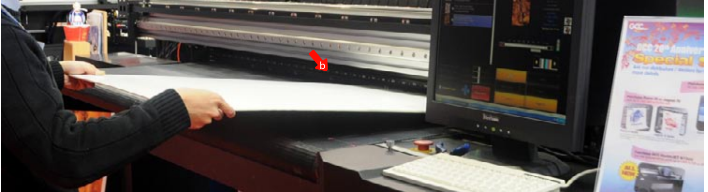
Media is aligned against a registration bar (b) that is moved up and down via software.
