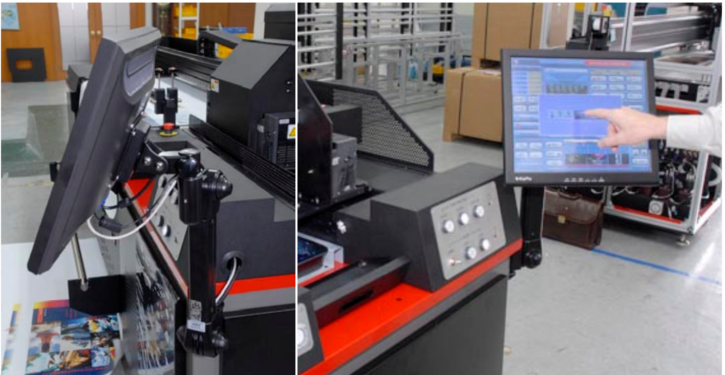
IP&I Cube 1606 at factory. The LCD monitor is attached to the printer but its angle can be varied by the operator.
