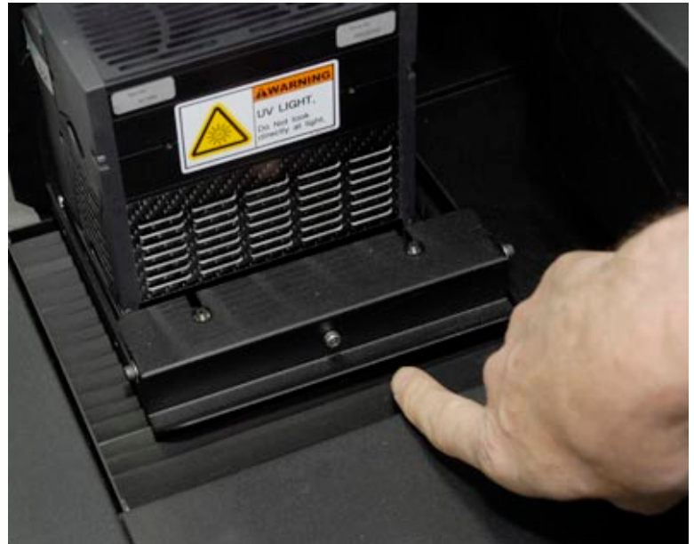
IP&I Cube 1606 at factory. An anti-head crash system, a bumper was one of the improvements made to the original model.
