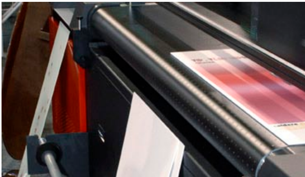
IP&I Cube 1606 at ISA 07. Materials are fed by a transport belt whereas the printhead carriage moves along the printing area
