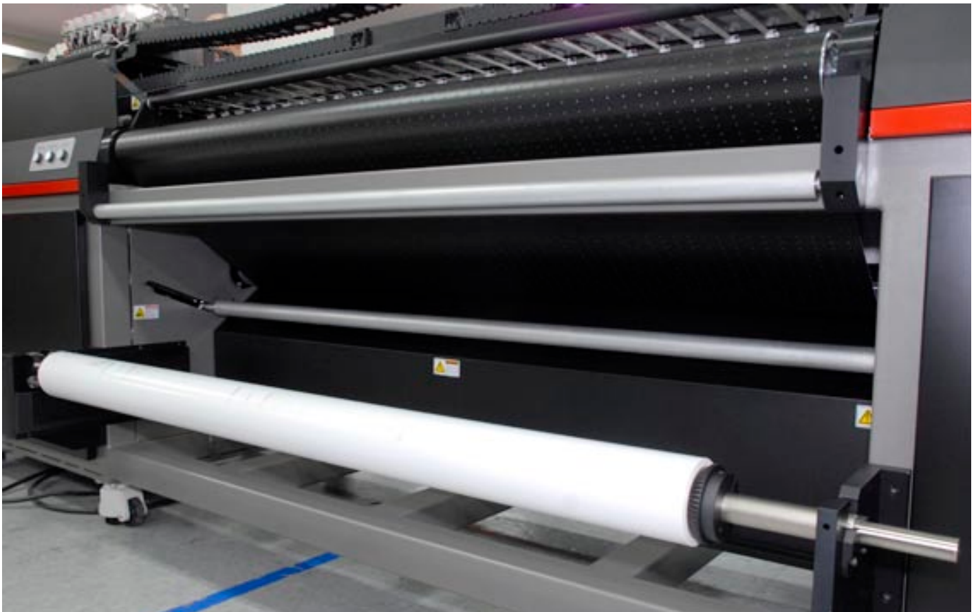
There are two rollers below the level of the transport belt: one is about 8" down, and a bit out in front. The dancer bar is about 50 cm inside and below. This is a unique system.
