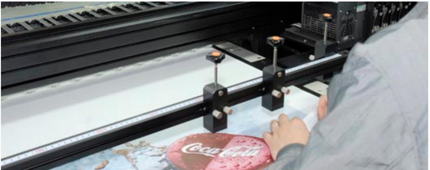
Measuring marks are used to attach rigid materials to the transport belt
