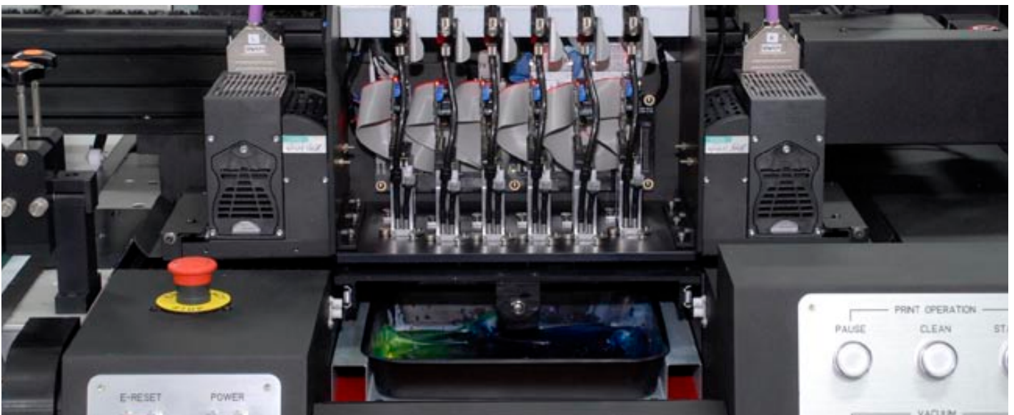
A drip tray collects the ink at right in the parking area
