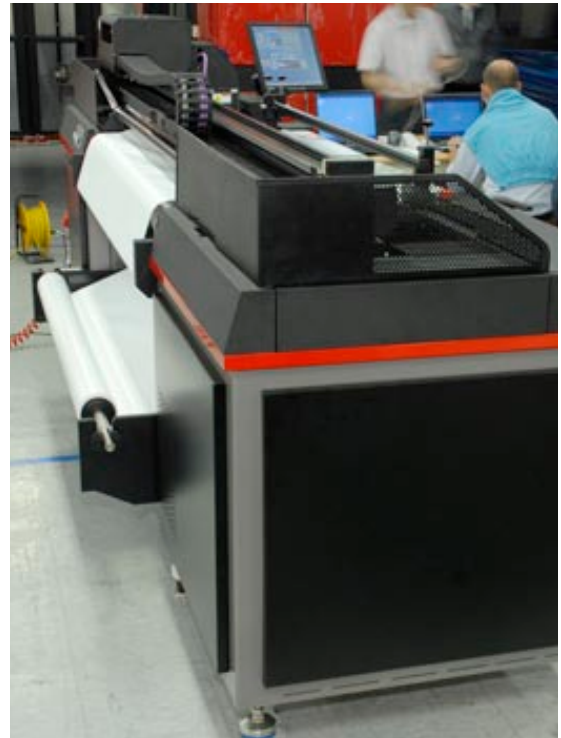
The spindle accepts 2" and 3" roll cores. But adapters are available.
