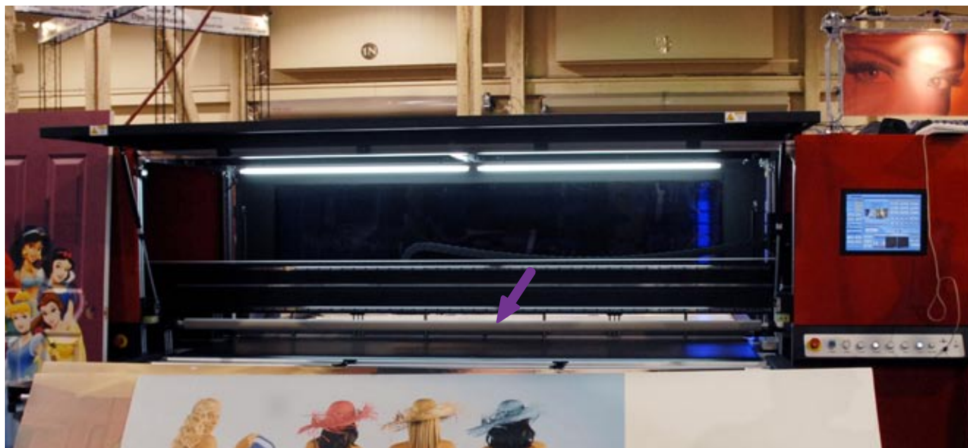
IP&I Cube260 at ISA 2007. A long pinch roller is placed across the front and another across the back of the printing area
