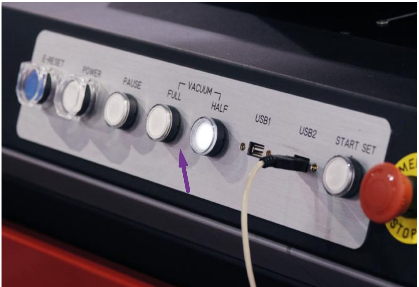
IP&I Cube260 at the manufacturing plant. You can see the two levels of the vacuum system, "FULL" and "HALF"
