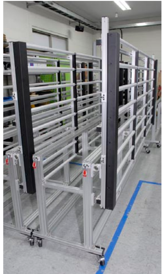
The flatbed table is not physically attached to the body of the printer. As you can see, the table consists of three sections of parallel rollers
