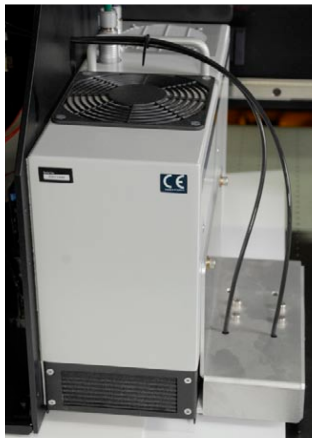
UV curing lamps from Integration Technology are placed at the sides of the printhead carriage
