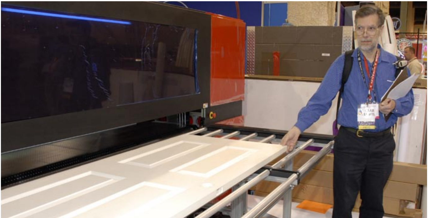
IP&I Cube 260UV. A door is being lined up to be printed. This model can print materials up to 3.75" (9cms) thick.
