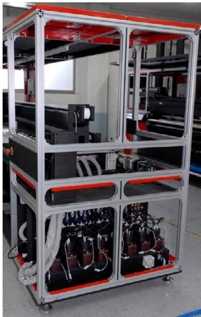
All ink containers are located at the left side, placed in one single row
