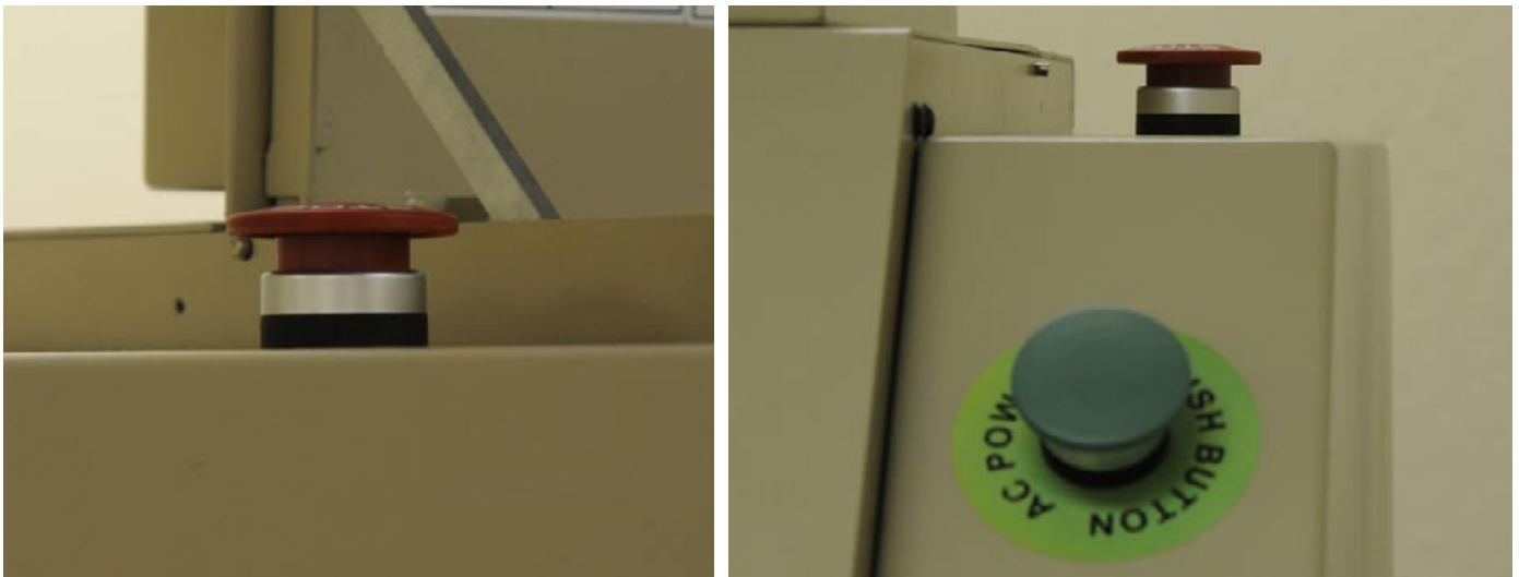
There is an emergency stop button at each end of the printer.
