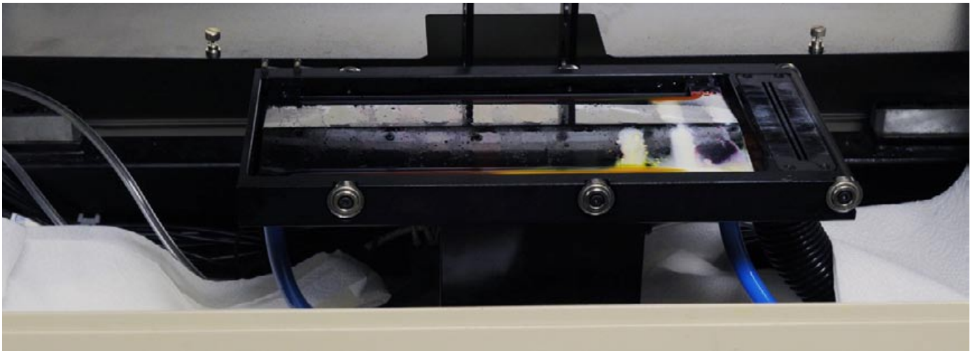
This tray receives the ink that is purged out of the printheads.
