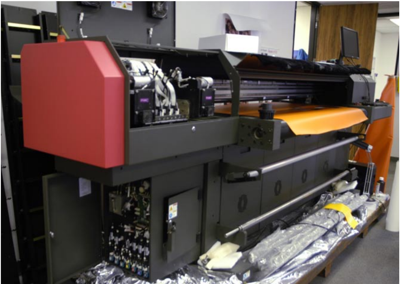
Cleaning station can be easily accessed. It is at the left. Here the printer at EFI Rastek headquarters in San Jose California.
