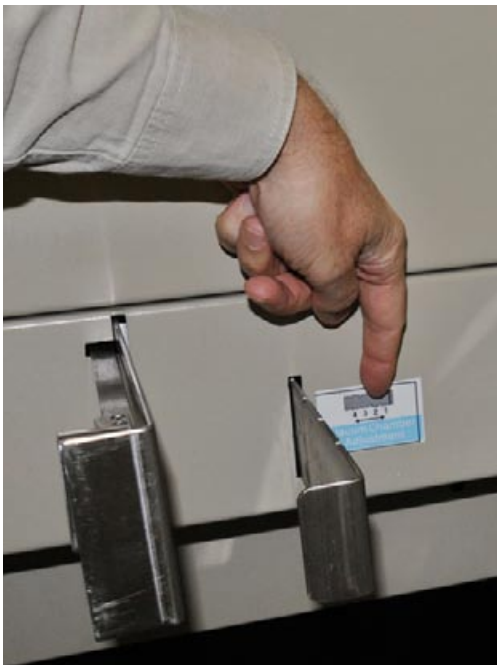
This is the handle to control the vacuum areas.
