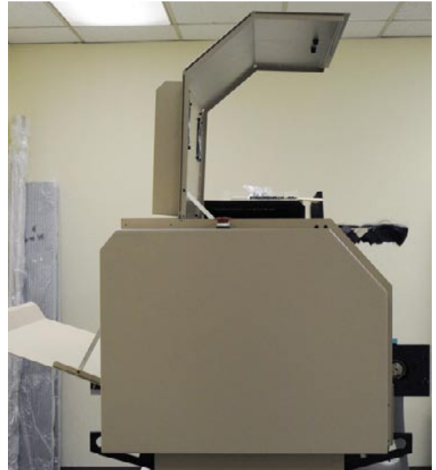
This is the hood of the service station.
