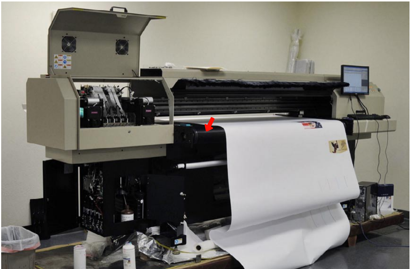
The machine has a transport belt; FLAAR classifies the H700UV as a Combo Printer.
