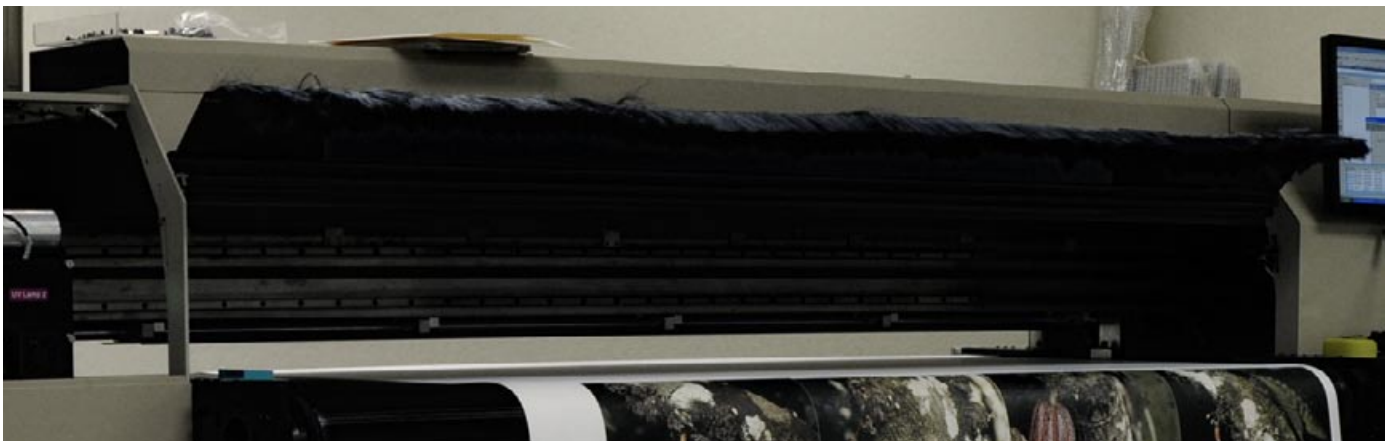
There is only one hood at front. No back hood was designed in the H700
