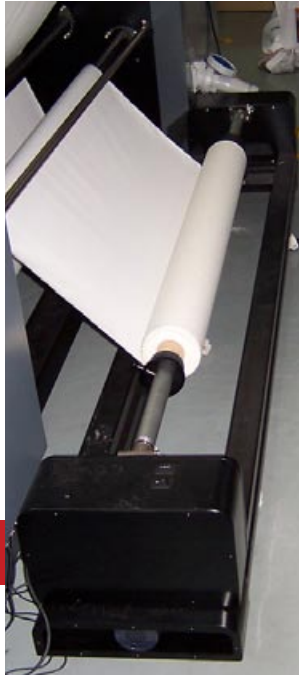
The take-up system and the feeding system can be detached and rolled away.
