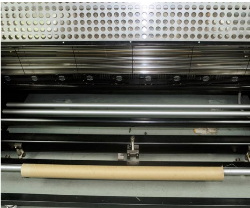
This is a solid machine that counts with an ample heater stretches across the entire front of the printing area.
