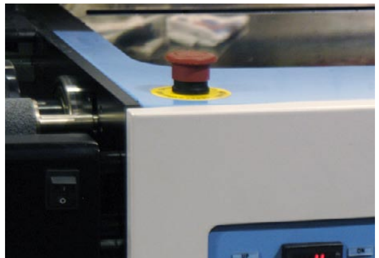
Emergency stop buttons are in the front, at each side of the printing area.
