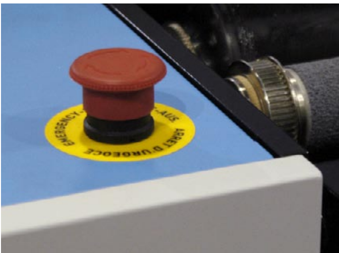
Emergency stop buttons are in the front, at each side of the printing area.
