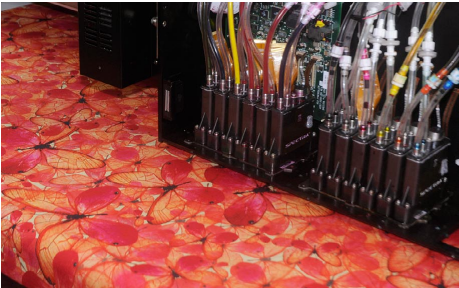
Yuhan K2 VU-1800 printheads and printed sample.
