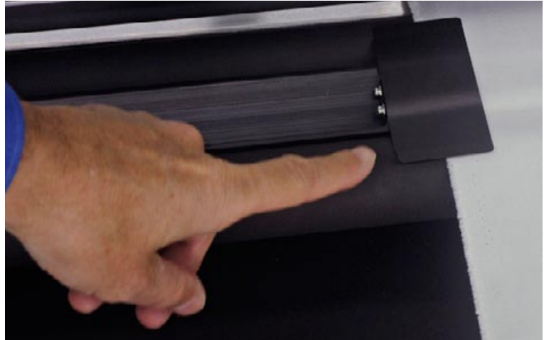
Edge guard. Since you are going to print different widths, these guards are movable.
