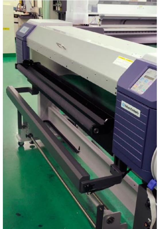
Heater unit is in the front.
