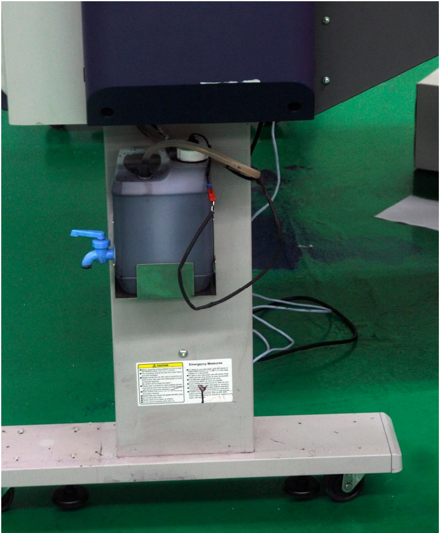
Waste ink container is at the lower right end of the printer.
