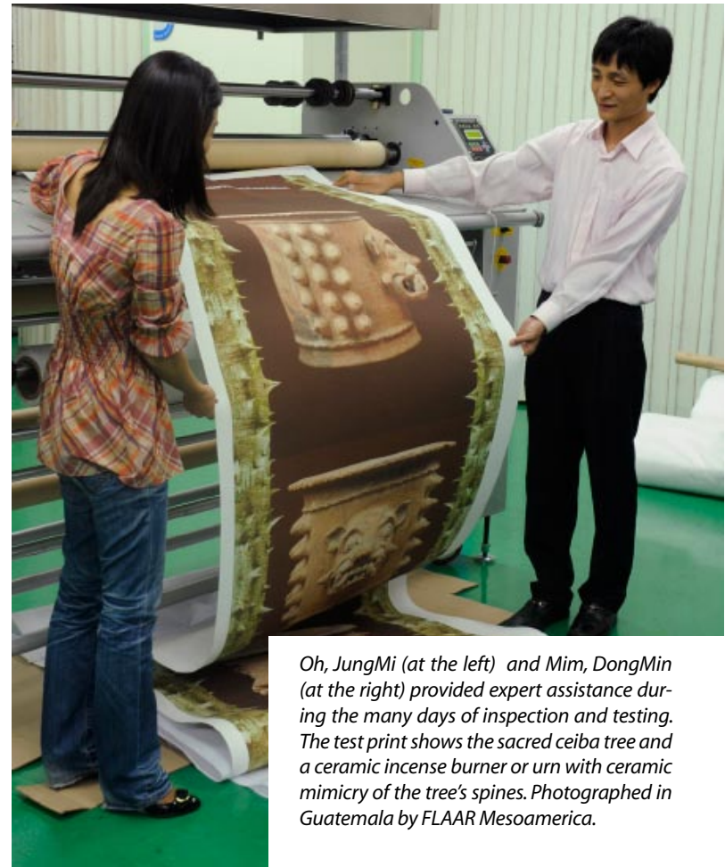
Comparing the colors before and after heat treatment. The color becomes more yellow after setting with heat. So the colors have to be tweaked to take this into account to begin with.
