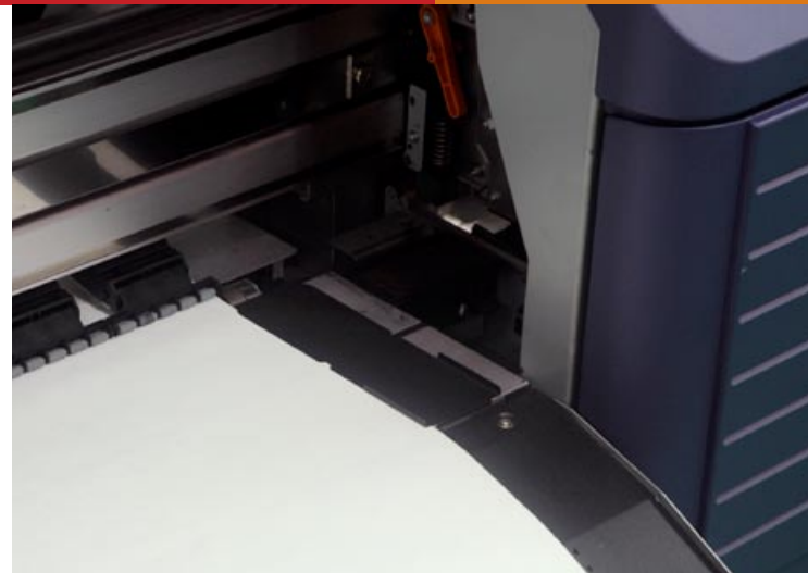
Showing the edge guard at the right. You can see two units of the pinch rollers, each with five gray rollers.
