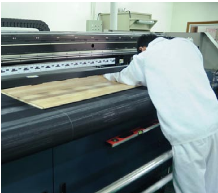
Wood boards being aligned to be printed on. Tong Jou Chemical also manufactures pretreatment liquids for wood.
