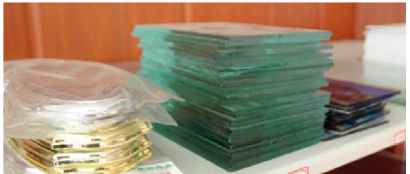
Media is any material that will be printed on. Glass usually requires treatment so that the ink will adhere to its non-porous surface.
