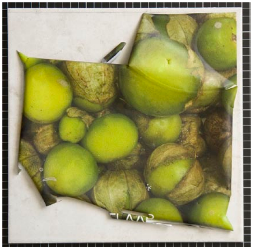
This floor tile printed on with a dedicated flatbed did not get the adequate pre-treatment. Imagine you print 1000 floor tiles for a thematic park in Florida without being aware of the need of treatment!
