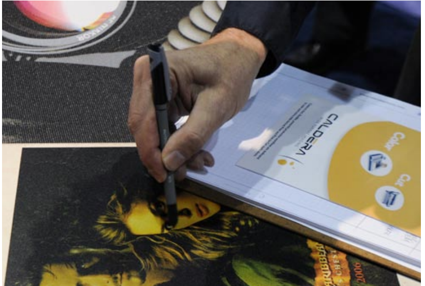
You can check the abrasion resistance yourself by scratching a print sample.
