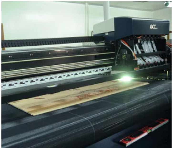
Wood boards being aligned to be printed on. Tong Jou Chemical also manufactures pretreatment liquids for wood.
