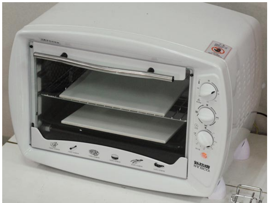
This is the drying unit used to fix the primer on tiles that will be printed on with the GCC StellarJET 250UV at Print in One sign shop, Taiwan.
