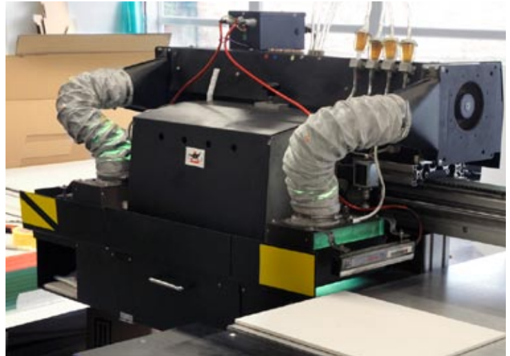
The capping station is in the same place as the parking station. Cleaning is also done here.
