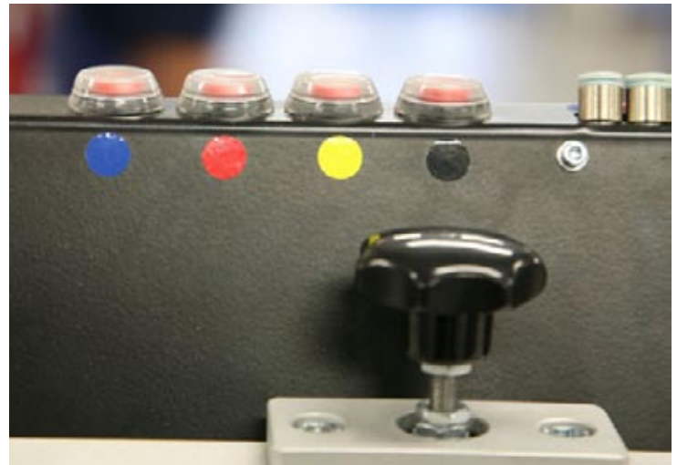
The purge has to be manual using buttons from each color.
