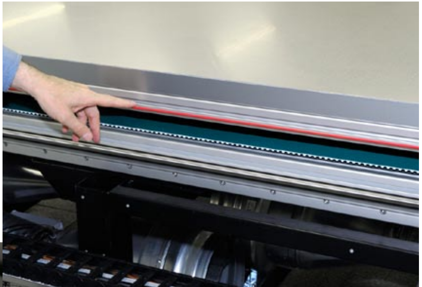
Above, you can see the emergency stop rope. This system is becoming popular among industrial size UV printers.
