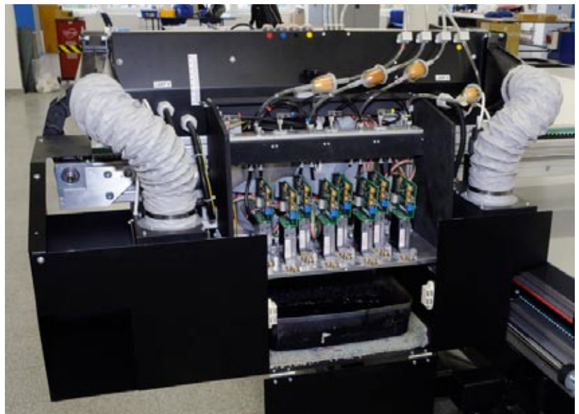
You should lower the heads into a soaked cloth to maintain the heads.
