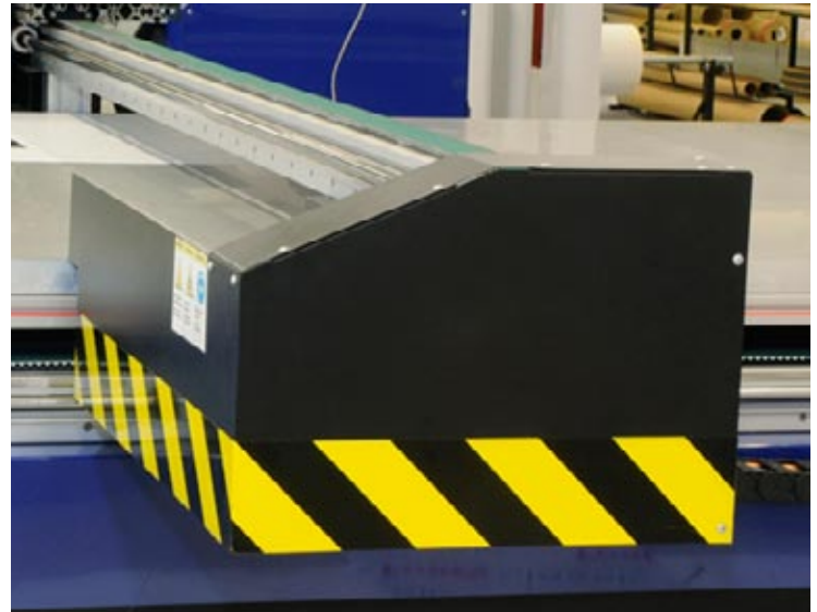
Not many printers have a means of warning people of moving parts that might hit a person. The only similar feature on other printers is the beacon light on the Dilli printers, but these only tell you that the printer is functioning.
