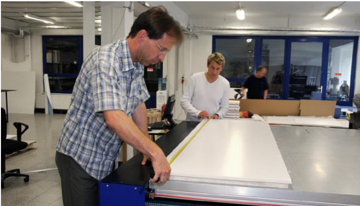
Because the printer has eight sections for vacuum, it is possible to print relatively small materials. Measuring materials is a manual task.
