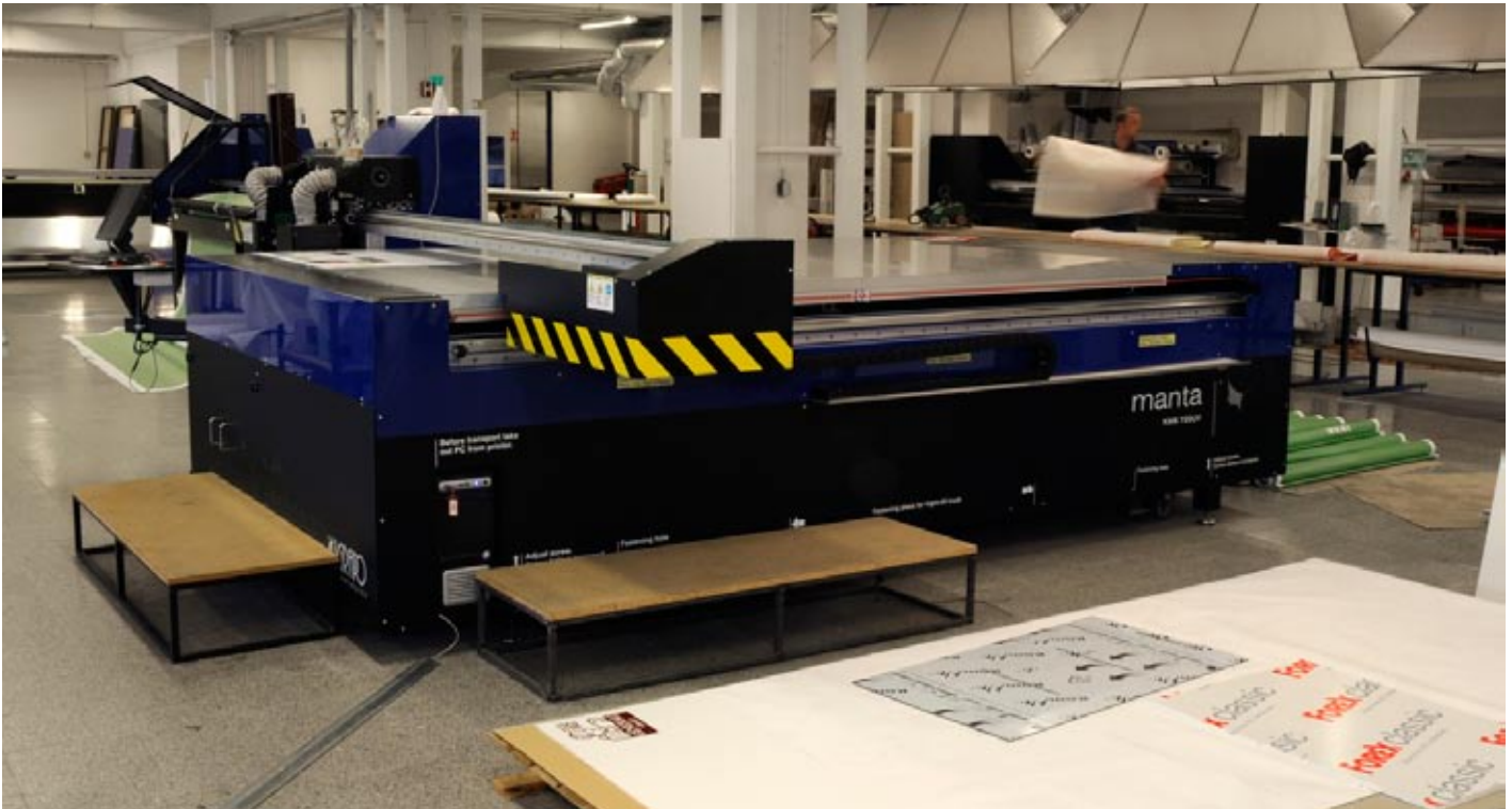
The flatbed table is stationary. What moves is the bridge where the carriage moves.
