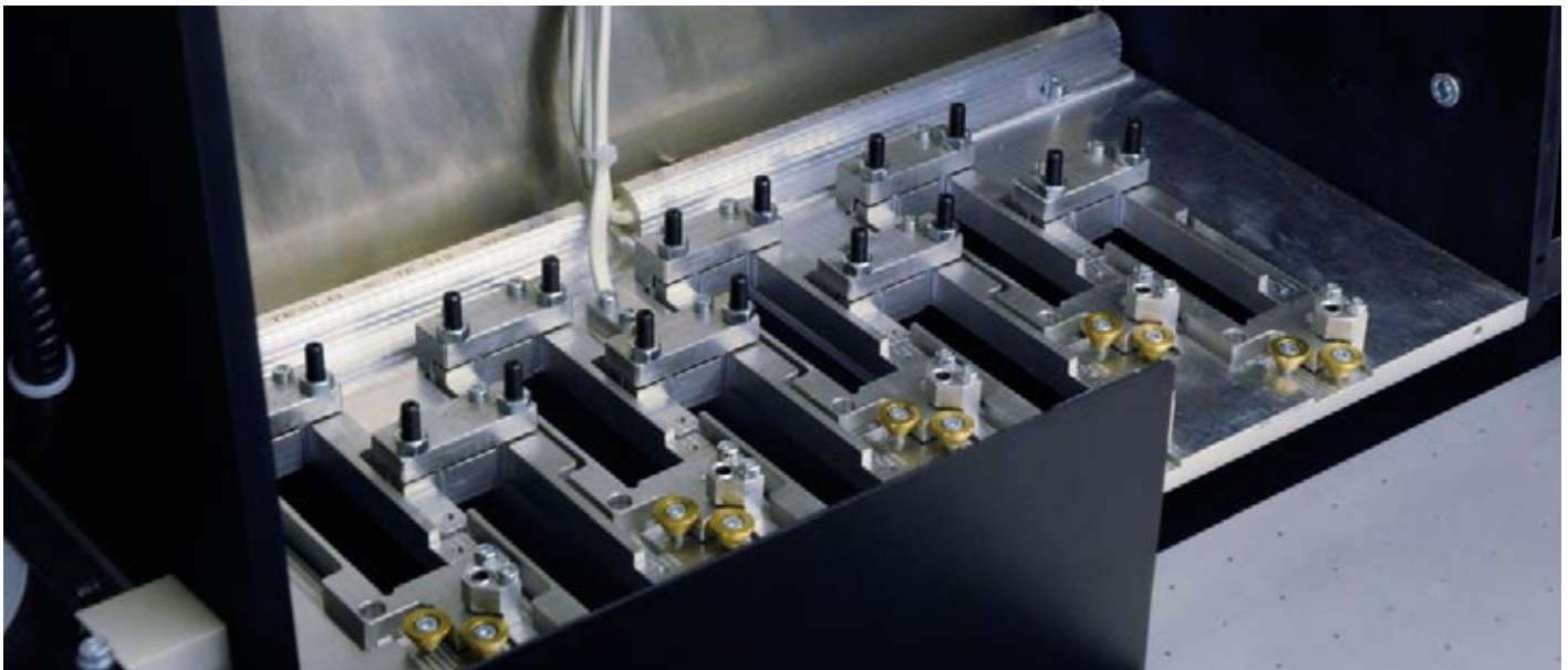
As you can see in the base plate, the printheads are staggered.
