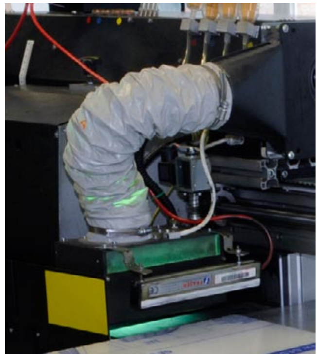
The Manta uses two industrial UV lamps.
