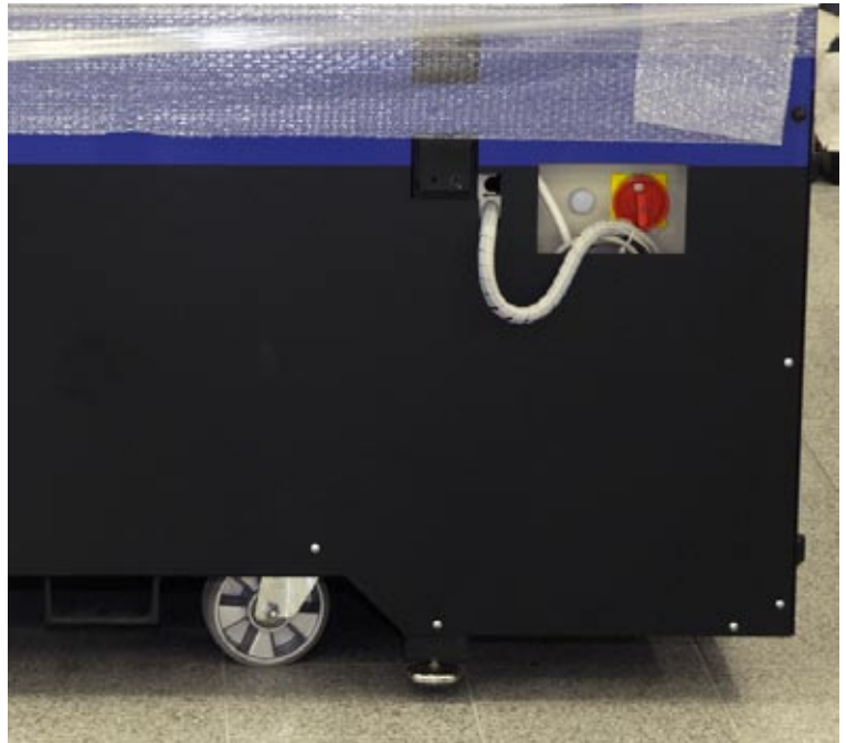
The Grapo Manta has four wheels and leveling supports.
