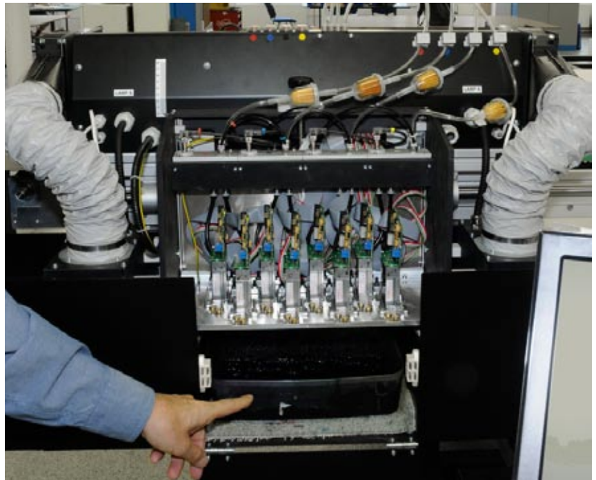
Ink that is purged goes into a drip tray.
