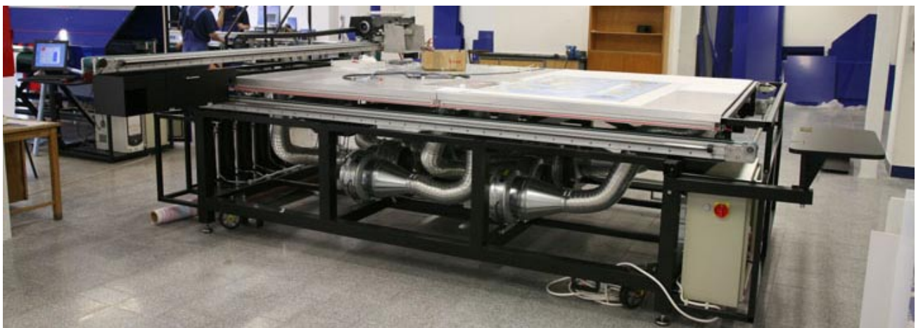
Below the flatbed table you can see the eight vacuum pumps.
